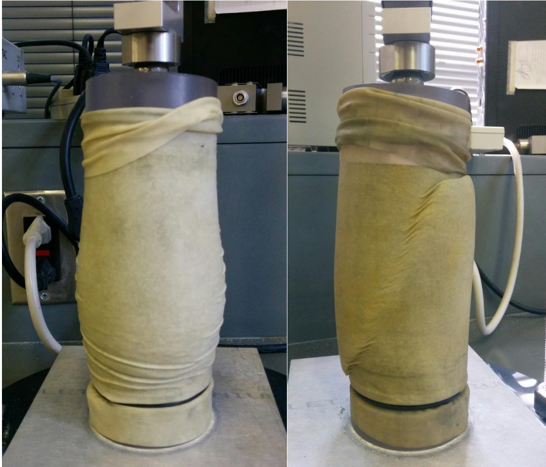
Figure B.3 Example of a loose sample (left panel) and a dense sample (right panel) failed in vacuum triaxial tests.
