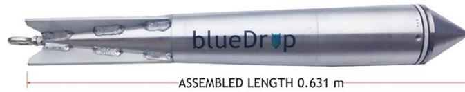
Figure 5.2. The FFP BlueDrop (modified from www.bluecdesigns.com ).
