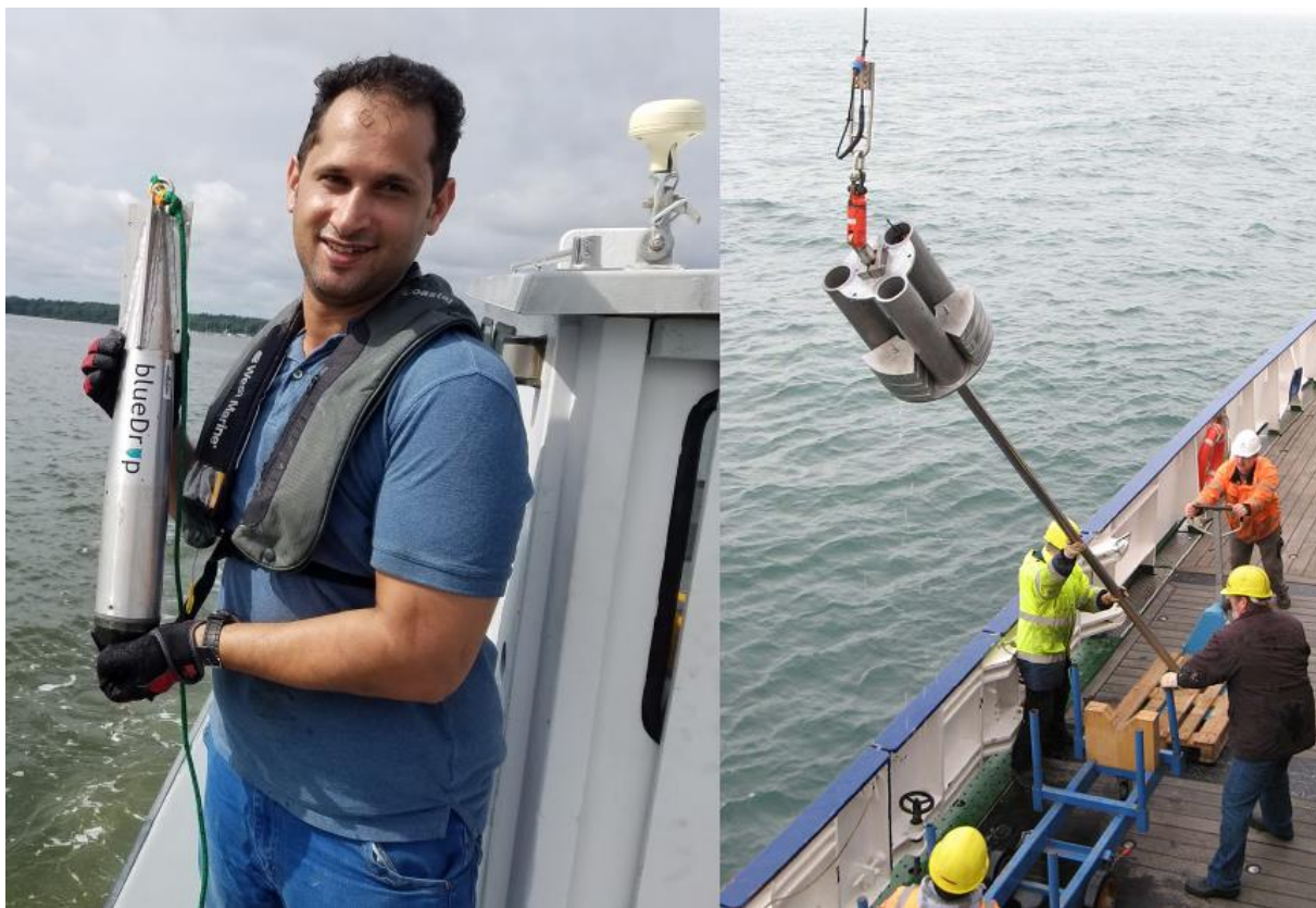
Figure 1.2. The projectile-like free fall penetrometer BlueDrop (left image), b) the lance-like free fall penetrometer LIRmeter (right image) (from: http://www.geo.uni-bremen.de ). The images also show the size and then required personnel to handle the device.
