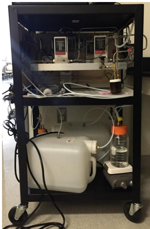
Figure B.20. The photo of the homemade humidity controller.
