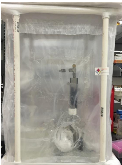
Figure B.19. Photo of the commercial atomizer contained in a homemade humidity chamber.
