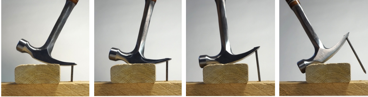
Figure 5.15 Use of a block of wood to alter the leverage for pulling nails with a rip claw hammer. Image: author.
