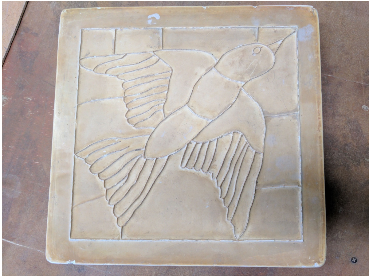
Figure 3.35. Plaster mold for bird tile mosaic, Moravian Pottery. Image: author, courtesy of the Moravian Pottery.
