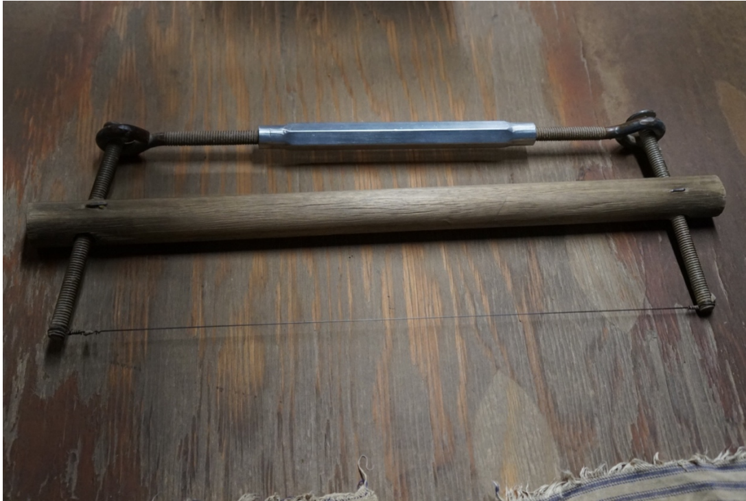
Figure 3.39. Wire “bon” for clay cutting, present day Moravian Pottery and Tileworks. Image: author, courtesy of the Moravian Pottery.
