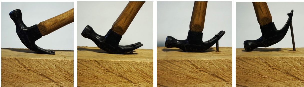
Figure 5.14 Diagram of the pulling of a nail with the finish hammer, which might be considered the paradigmatic case of the geometry of the tool optimized to provide for a primary design function. Note that the geometry of the curved claw provides for a stable point of rotation of the hammer, such that the user can maintain a high ratio of mechanical advantage throughout the process of pulling the nail. Image: author.
