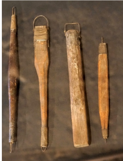
Figure 3.41. Loop tools from the early years of the Moravian Pottery. Image: author, courtesy of the Moravian Pottery.
