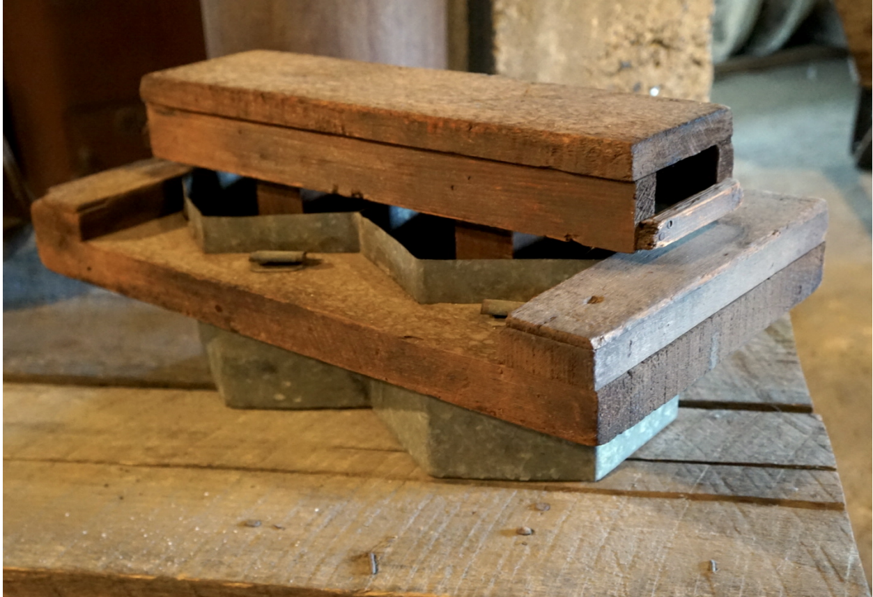
Figure 3.27. Hexagonal tile maker, Moravian Pottery. Image: author, courtesy of the Moravian Pottery.
