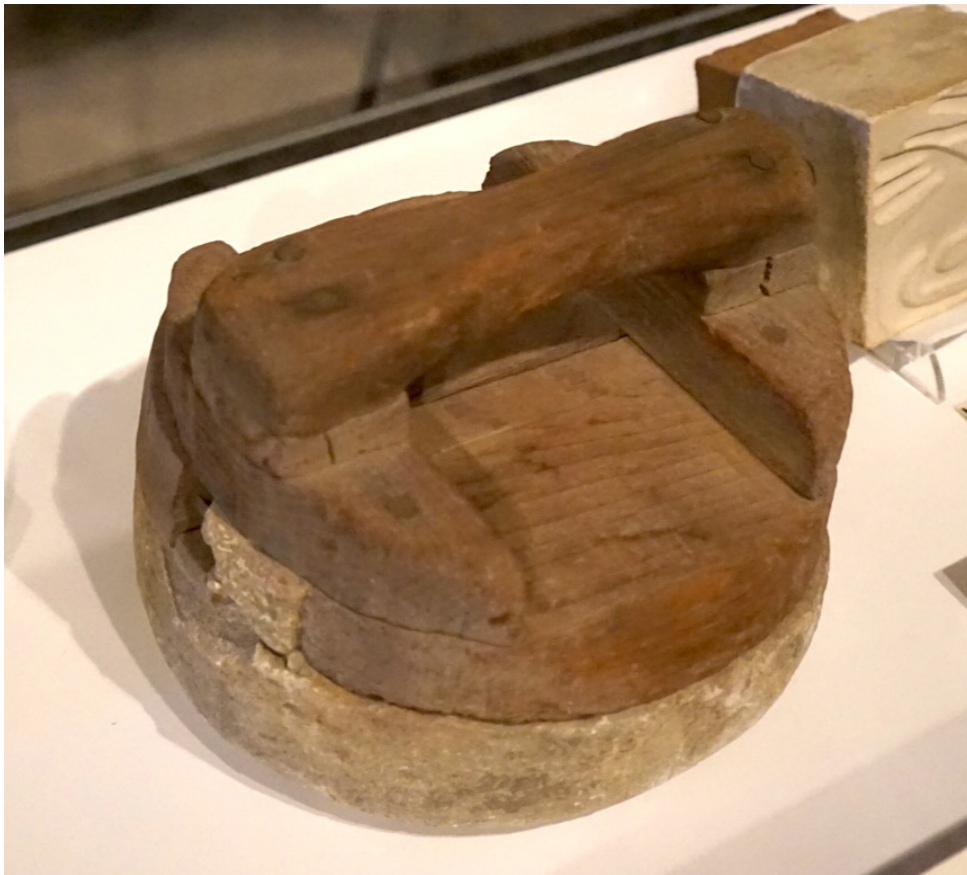
Figure 3.31. Wooden hand-held clay pressing tool. Image: author, courtesy of the Moravian Pottery.
