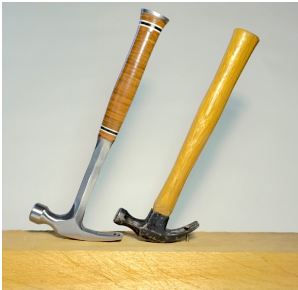
Figure 5.12 Two common types of carpenter's hammer, the rip claw or "framing" hammer, and the curved claw, or "finish" hammer. Despite their common names, both types of hammers are used, at times interchangeably, in the work of both rough and finish carpenters. The differences between the two relate to the overall weight of the hammer—a framing hammer is heavier, between 22 and 24 ounces, versus the finish hammer's 16-20 ounces—and the curvature of the claw. Image: author.
