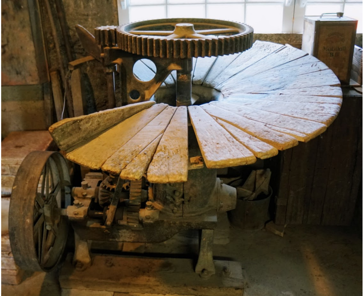
Figure 1.4. Historic pugmill, no longer in use, at the current site of the Moravian Pottery. Image: author, courtesy of the Moravian Pottery.
