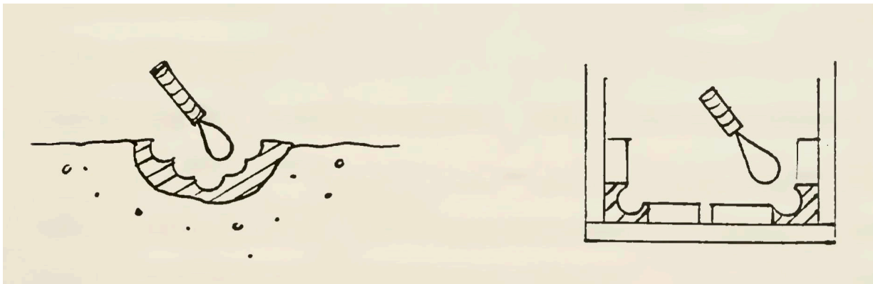
Figure 3.40. Walsh's drawing of the tool used to create the beaded beams in the 'saloon' room at Fontbill. Image: Marianne Walsh, Finishes Analysis in the Saloon, Fontbill.
