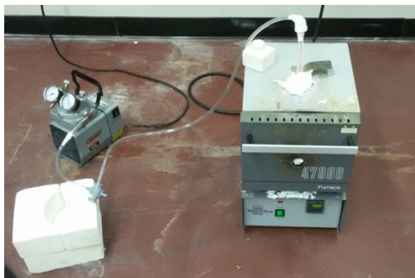
Figure 86: YBCO/SiO 2 tube sample inserted vertically inside the furnace
