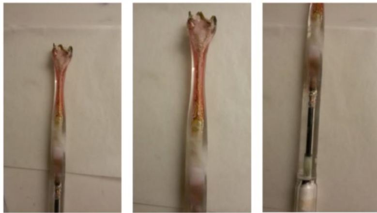
Figure 23: YBCO preform after a blow-out
