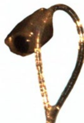
Figure 31: YBCO core fragment mounted with Paratone oil on a Nylon loop
