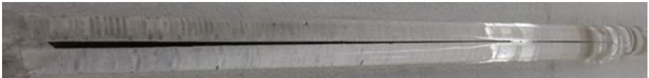
Figure 19: Tapered preform with YBCO powder
