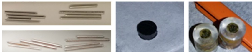
Figure 94: Illustration of the three main focus areas of this dissertation: reactions within YBCO glass fibers (left), reactions within YBCO+SiO 2 pellets (middle) and rapid thermal annealing experiments on YBCO-SiO 2 samples (right, showing a thermally annealed and quenched YBCO/SiO 2 tube)
