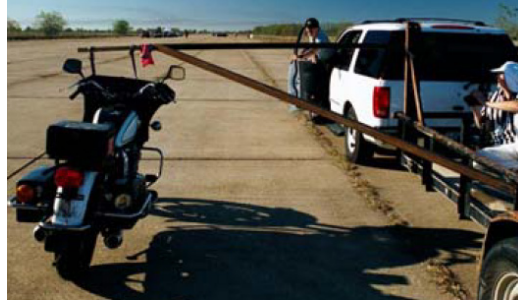
Figure 32. Motorcycle tow system (Adamson et al., 2002).
