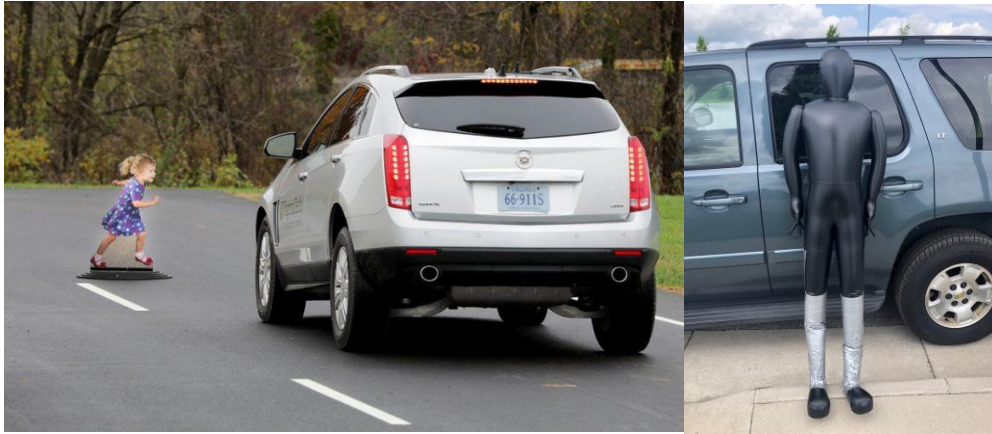
Figure 11: HV-REMO base on the Smart Road with a pedestrian cardboard cut-out attached (left). Soft target attachment used for this project (right).
