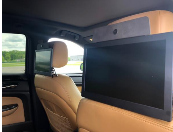
Figure 4: Video screens installed for HMI conditions.
