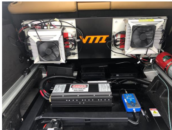
Figure 5: Data acquisition (top-left silver box) and automation system (remaining added components) installed into the trunk of the test vehicle.
