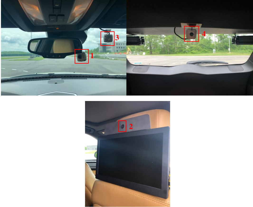
Figure 6: Camera positions for capturing participant face-views (1 & 2), the roadway (3), and screen-view video (4).
