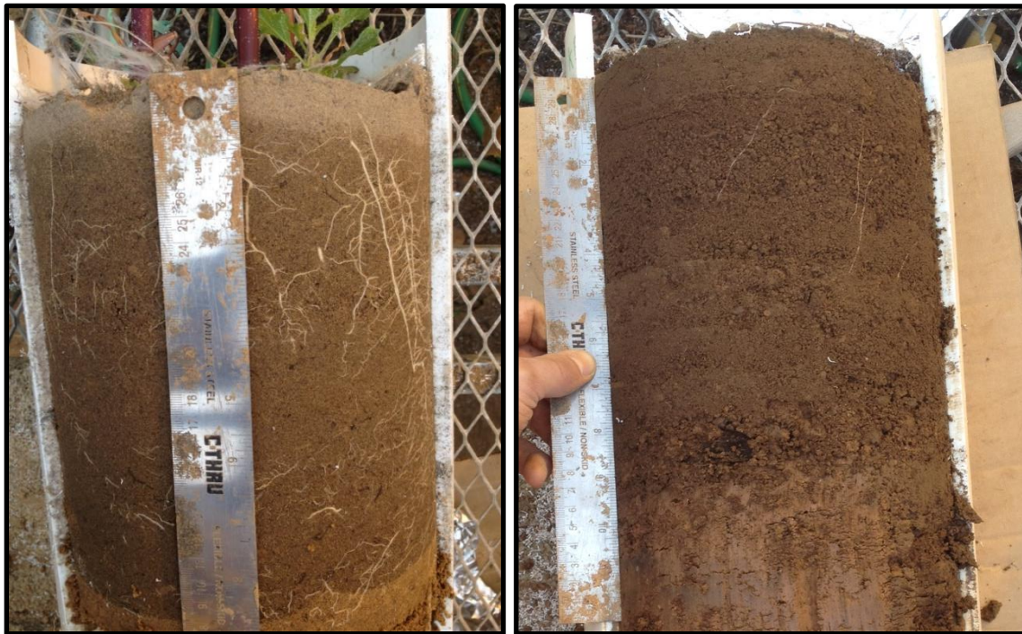
Figure A4. “sand” (left) vs “loam” (right) soil columns (60 cm) cut longitudinally. Notice the layer of dry soil on the surface of the sand column, indicating higher ET (compared to loam columns) throughout the experiment.
