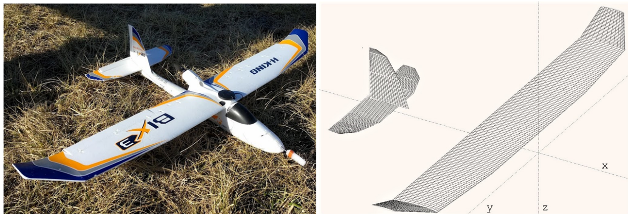
Figure 3.3: Bix3 aircraft (left), and the XFLR5 model of the Bix3 wing and tail (right)
