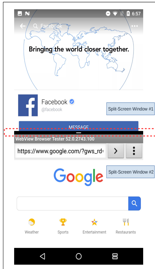
Figure 3.1: A screenshot of split-screen execution in Android Nougat, where the top window runs Facebook while the bottom window simultaneously runs a web browser. The dimensions of the split-screen can be altered by dragging the black bar separating the two windows.
