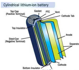
Fig 2. Parts of a lithium-ion battery [3]
