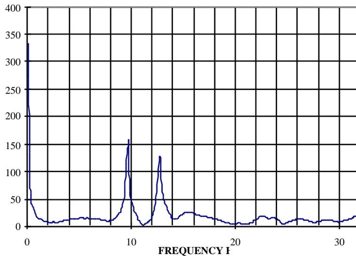
**Figure 2.13 Power Spectrum Showing Two Frequencies of Vibration**
