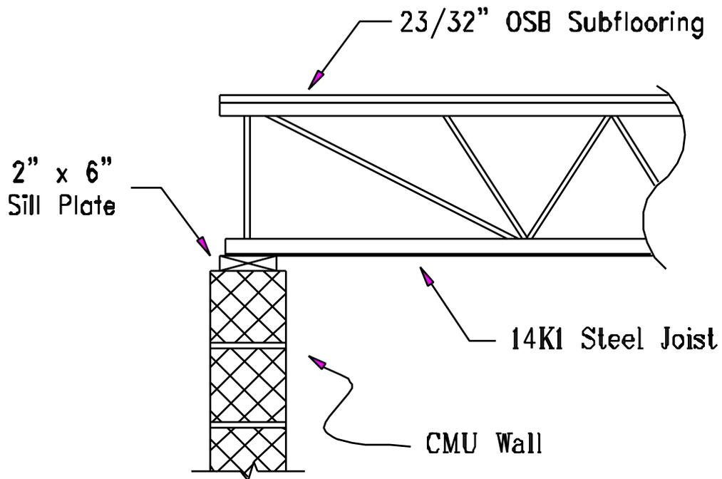
Figure 2.2 Section A-A from Figure 2.1
