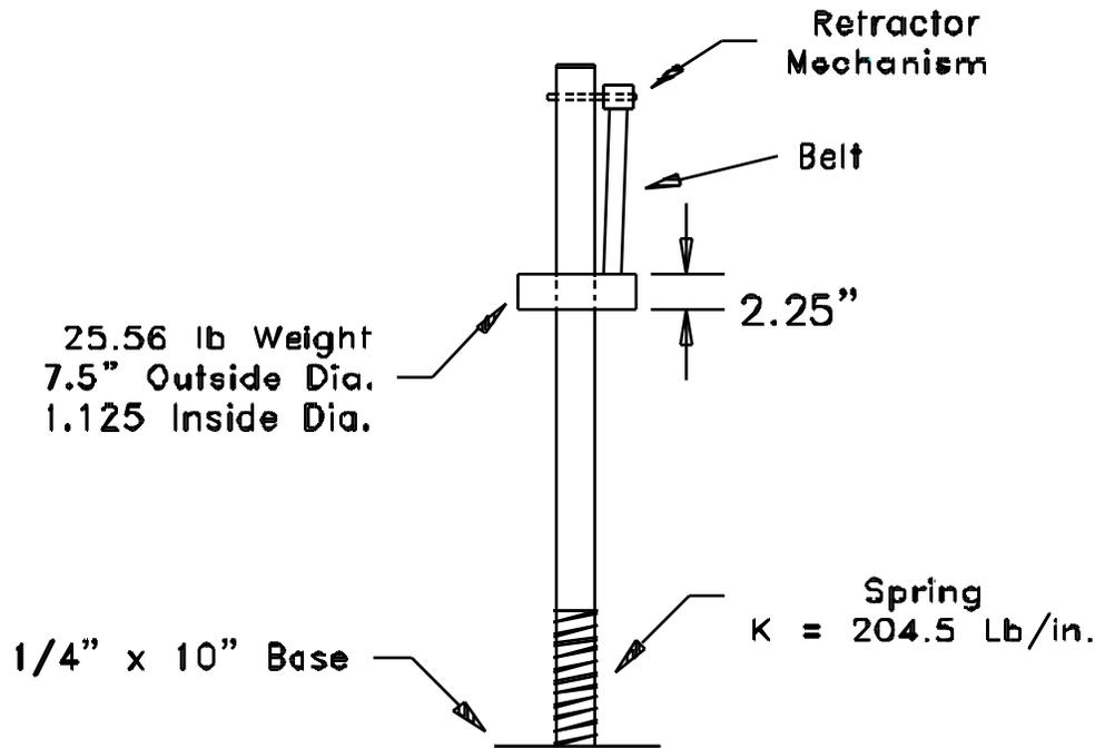
**Figure 2.5 Heel Drop Simulator (HDS) Machine**
