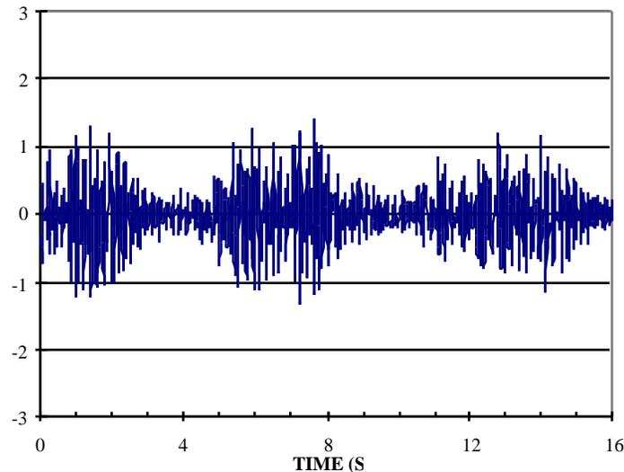
**Figure 2.10 Example of a Walking Acceleration Trace**
