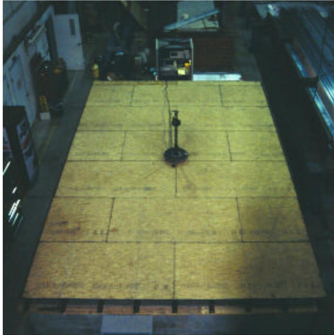
**Figure 2.6 HDS, Force Plate and Accelerometer Located at midspan of Floor**
