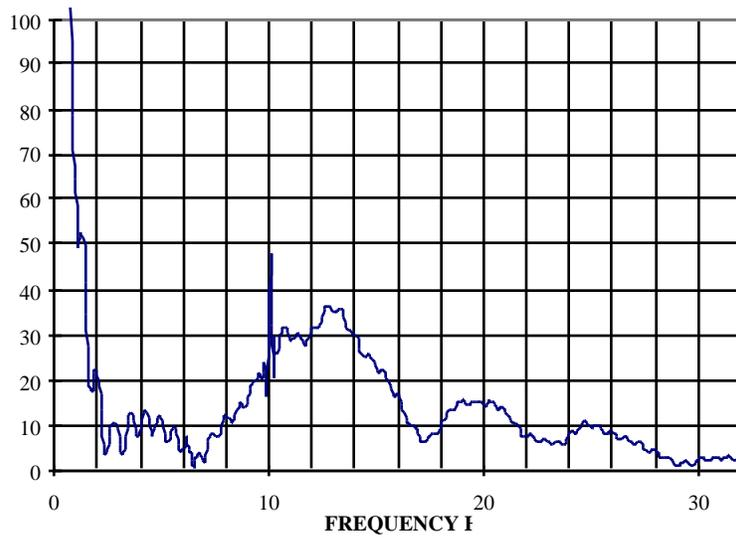
**Figure 2.15 Power Spectrum Showing Multiple and Torsional Modes of Vibration**
