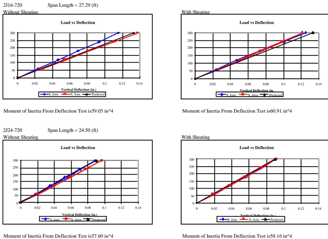
**Figure 2.12 Load versus Deflection Tests for Two-Joist Floor Systems**
