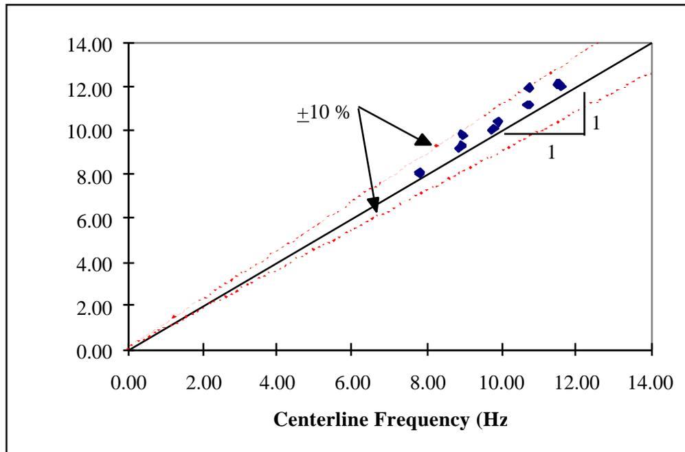
**Figure 2.14 Fundamental Frequency from Heel Drop Impact Tests at Different Locations: Quarter Point versus Midspan**
