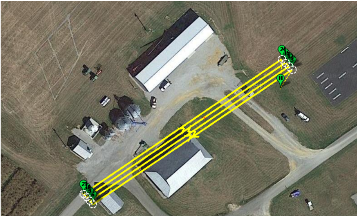
Figure 3.14: Lawn-Mower pattern flight plan to collect real data for algorithm testing
