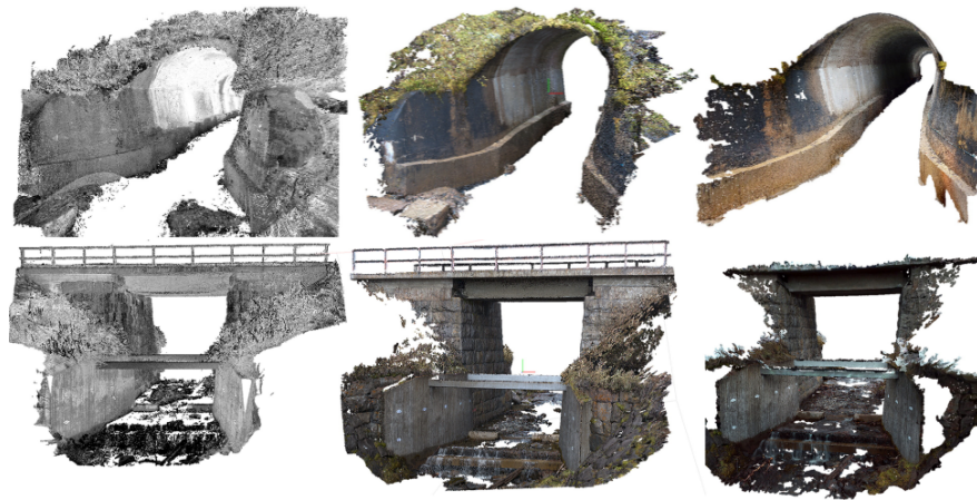
Figure 2.2: Comparison of laser, photogrammetry, and infrared sensing on two different scenes. Tunnel (top row) and bridge (bottom row). Laser ranging (left column), photogrammetry (middle column), infrared (right column) [18]
