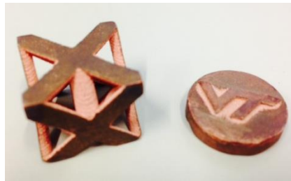
Figure 2.8 Complex shaped copper made via Binder Jetting
