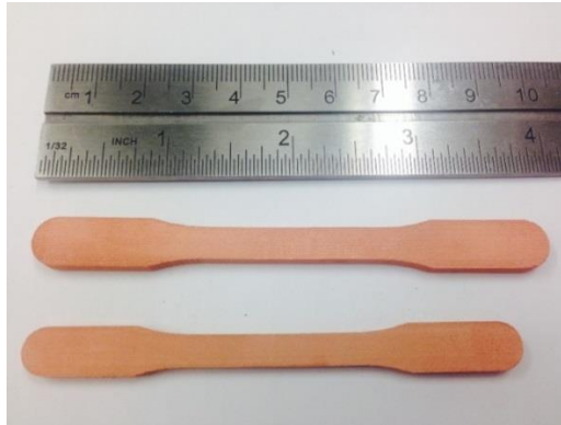
Figure 2.11 Tensile test specimen sintered at 1060 °C (top) and 1080 °C (bottom)
