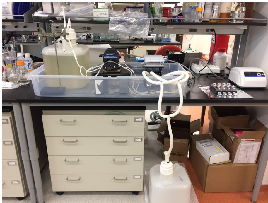
Figure 2-16. Sterilized Reactor System Ready for Batch Phase Growth
