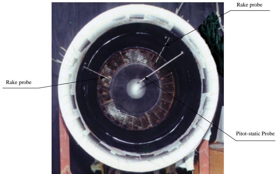
Figure 3.7: Frontal View of Probes for Mass Flow Measurement.
