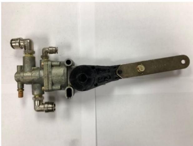
Figure 2.10: The chambered load leveling valve – assembled (left); components [14] (right)
