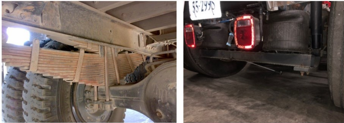
Figure 2.1: Leaf suspension in application [4] (left); Air suspension in application (right)
