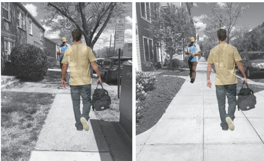
Figure 17. Sidewalk Widening. The Braddock Metro Neighborhood Plan specifies the widening of sidewalk pedestrian zones from typically four feet (left) to a minimum of six feet (right), enhancing accessibility and allowing for minimally restricted pedestrian movement.
