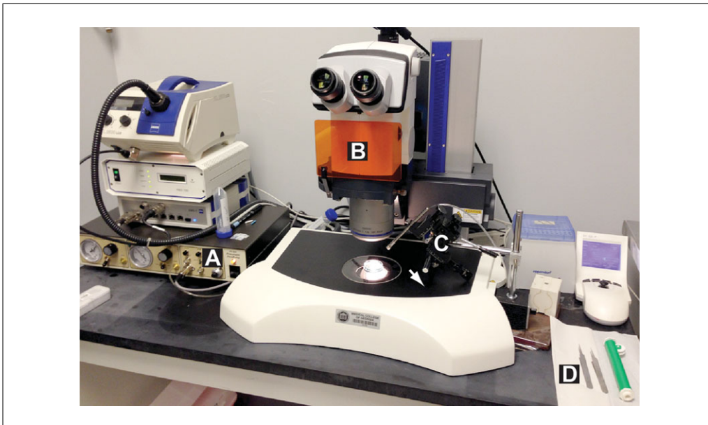
Figure 1.26.6 Zebrafish injection setup. (A) Pneumatic pump, (B) stereomicroscope, (C) micro-manipulator, and (D) forceps and pipette pump.
