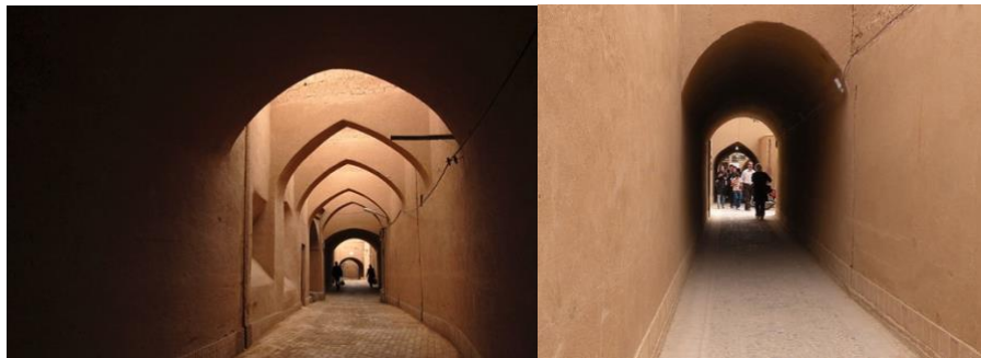
Figure 14. Yazd Alleys Are Built to Keep The Most Comfort to The Pedestrians by Casting Shadows and Most of Times Oriented to Conduct The Wind Flows
