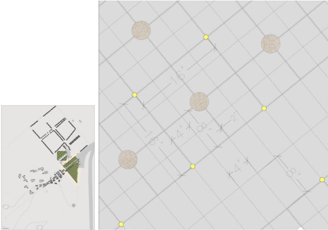
Figure 62. Material of Surface -Light Gray Concrete Slab with Gravel in Between
