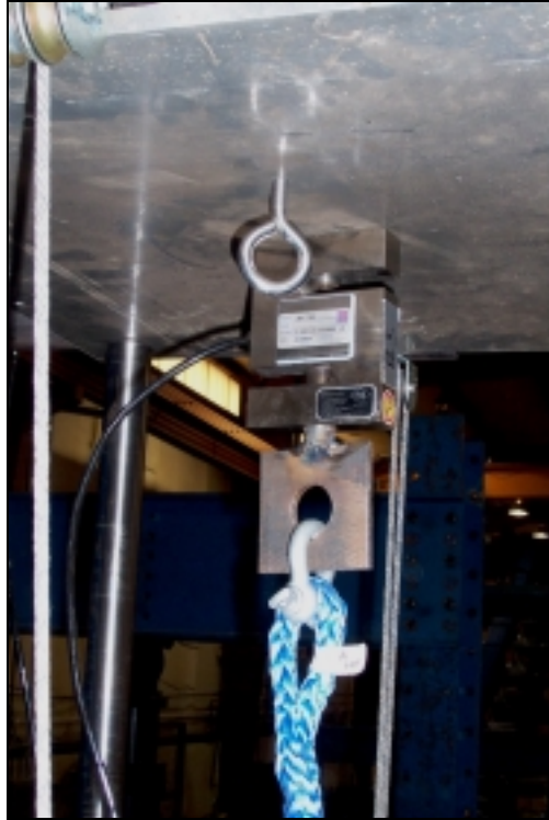
Figure 2.2.3: Photograph of the Load Cell Assembly
