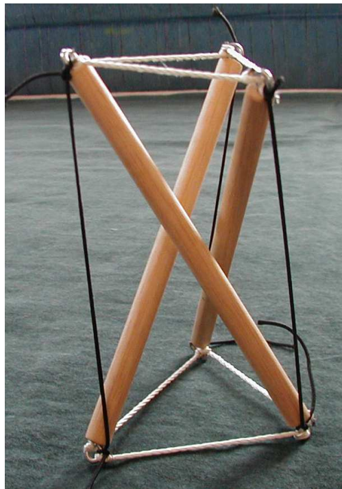
Figure 1.3: Example tensegrity structure [Whittier, 2002]
