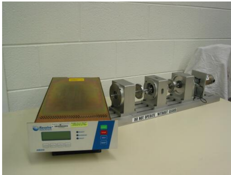
Figure B.1: Revolve MB350 and MBRotor Active Magnetic Bearing
