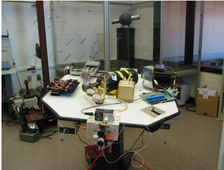
Figure A.1: Whorl-1 with Magnetic Bearing on Top Deck
