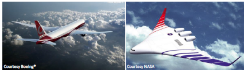
Figure 1.1. Modern aircraft 'tube-and-wing' design (Left) and future blended wing design (Right).
