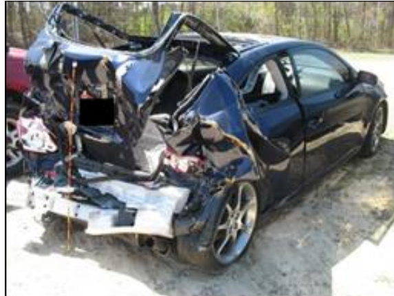
Figure 28. Fatal rear crash in which compartmental collapse resulted in the right rear passenger sustaining a fatal head injury. The driver and right front passengers sustained only minor AIS1 injuries in this crash (NASS-CDS 2010-43-051).
