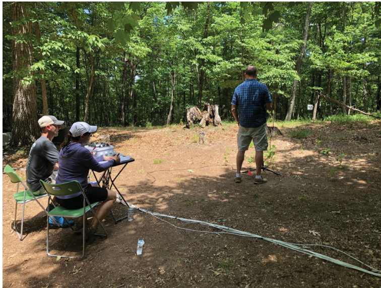
Figure . Field posttest site layout with participant standing in center of remote firing devices facing 12 o'clock target position and two investigators seated behind participant between the 6 o'clock and 7 o'clock positions.
