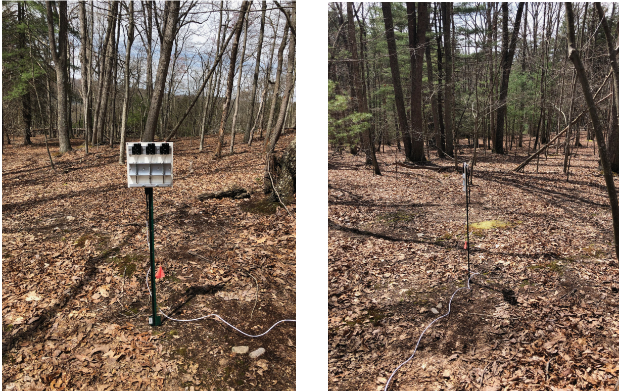
Figure . One remote firing device containing three remote firing mechanisms mounted on a steel u-post located in the wooded forest at the field localization site (Left: Front view of remote firing device, Right: Profile (side) view as seen from direction of the participant), which reduced the visual signature.
