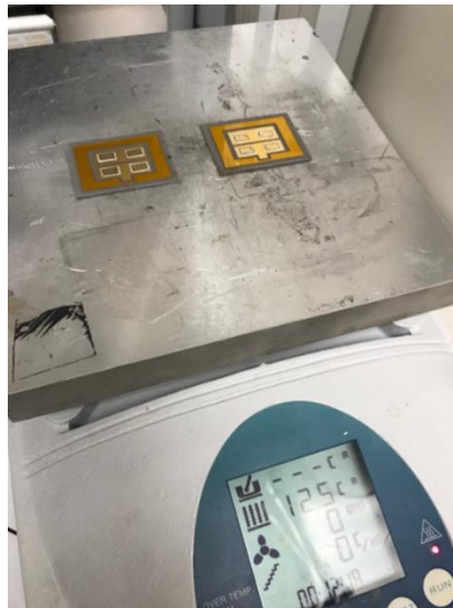
Figure 3-11. Substrate placed onto programmable hotplate
