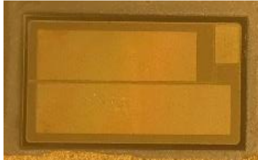
Figure 3-21. Die with nickel:gold topcoat and space around the gate terminal
