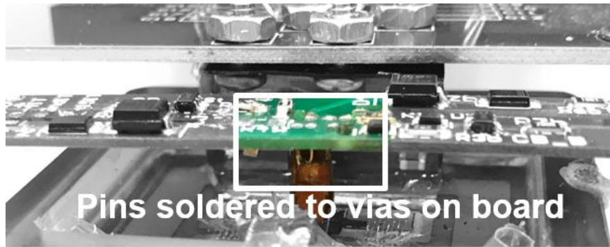
Figure 4-10. Pins of the flexible PCB interface with vias on the board
