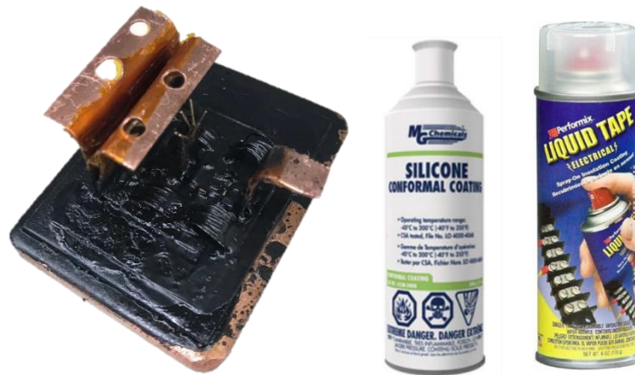
Figure 3-41. Module 9 alternative encapsulation technique for black surface IR camera compatibility
