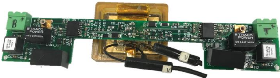
Figure 4-9. Gate driver with top and bottom switch circuitry designed to be thin for the placement of the Rogowski coils
