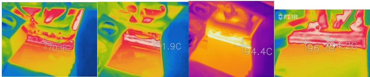
Figure 5-26. Thermal image of modules 4, 6, 8, and 9 at 200 V, 37.7 A input, 400 V, 18.85 A output
