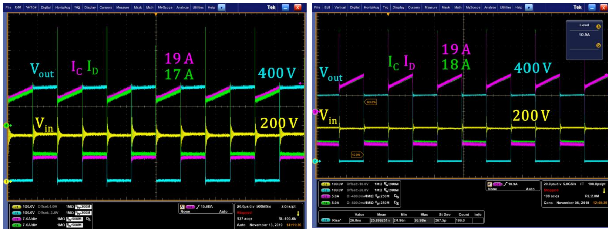
Figure 5-14. Continuous test results for balanced modules 4 and 6 at 200 V, 37.7 A input
