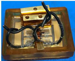
Figure 3-39. a. Two parts of encapsulant are mixed producing bubbles b-c. Bubbles are removed using a vacuum d. Encapsulant is poured into the module producing bubbles e. Bubbles are removed f. Encapsulant is cured at 70°C for 4 hours
