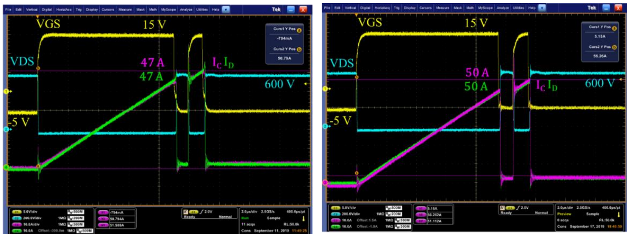
Figure 4-28. 600 V DPT results for balanced modules 4 and 6
