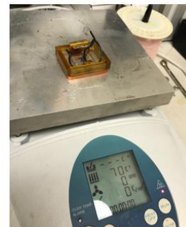
Figure 3-39. a. Two parts of encapsulant are mixed producing bubbles b-c. Bubbles are removed using a vacuum d. Encapsulant is poured into the module producing bubbles e. Bubbles are removed f. Encapsulant is cured at 70°C for 4 hours
