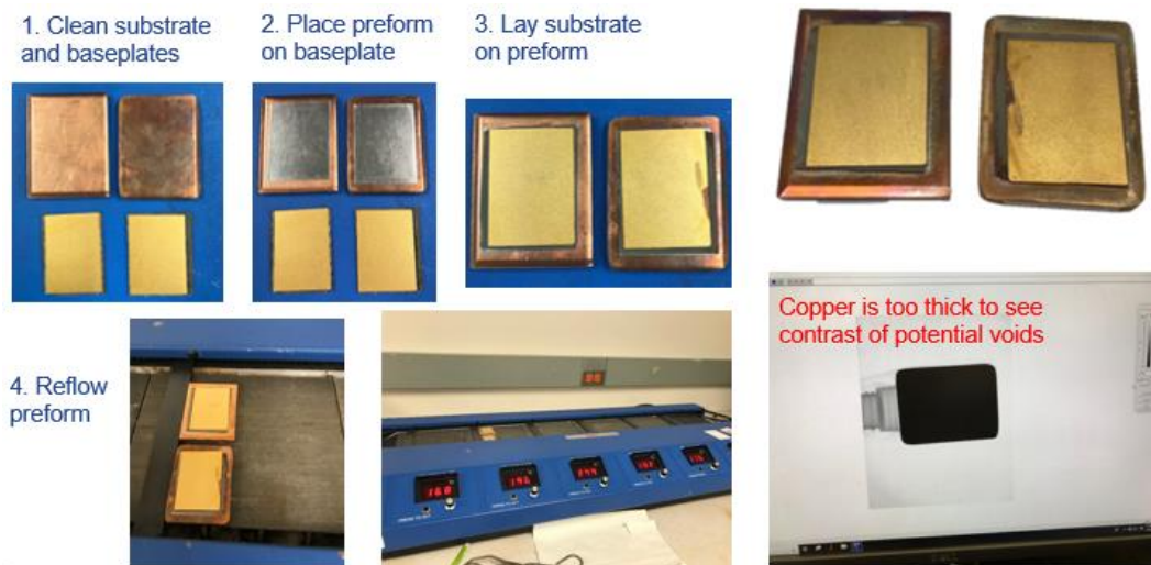
Figure 3-32. Solder preform sits between the baseplate and the DBC
