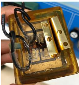
Figure 3-39. a. Two parts of encapsulant are mixed producing bubbles b-c. Bubbles are removed using a vacuum d. Encapsulant is poured into the module producing bubbles e. Bubbles are removed f. Encapsulant is cured at 70°C for 4 hours
