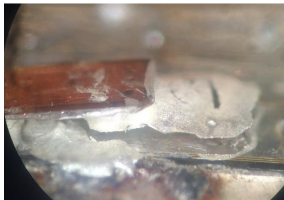
Figure 3-20. Microscopic image of sinter paste not adhering to aluminum surface of die
