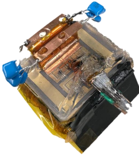
Figure 5-9. Fully fabricated module with heat sink and black liquid tape covering the face of the baseplate
