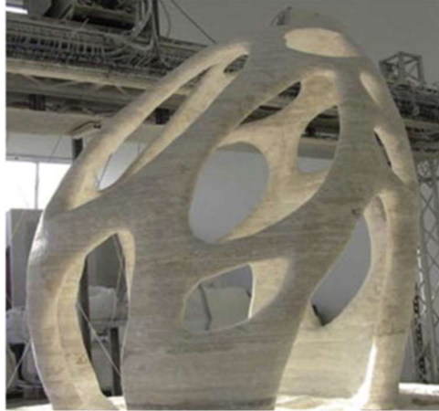
Figure 2.4: Example of D-Shape (from Lim et al. [8])
