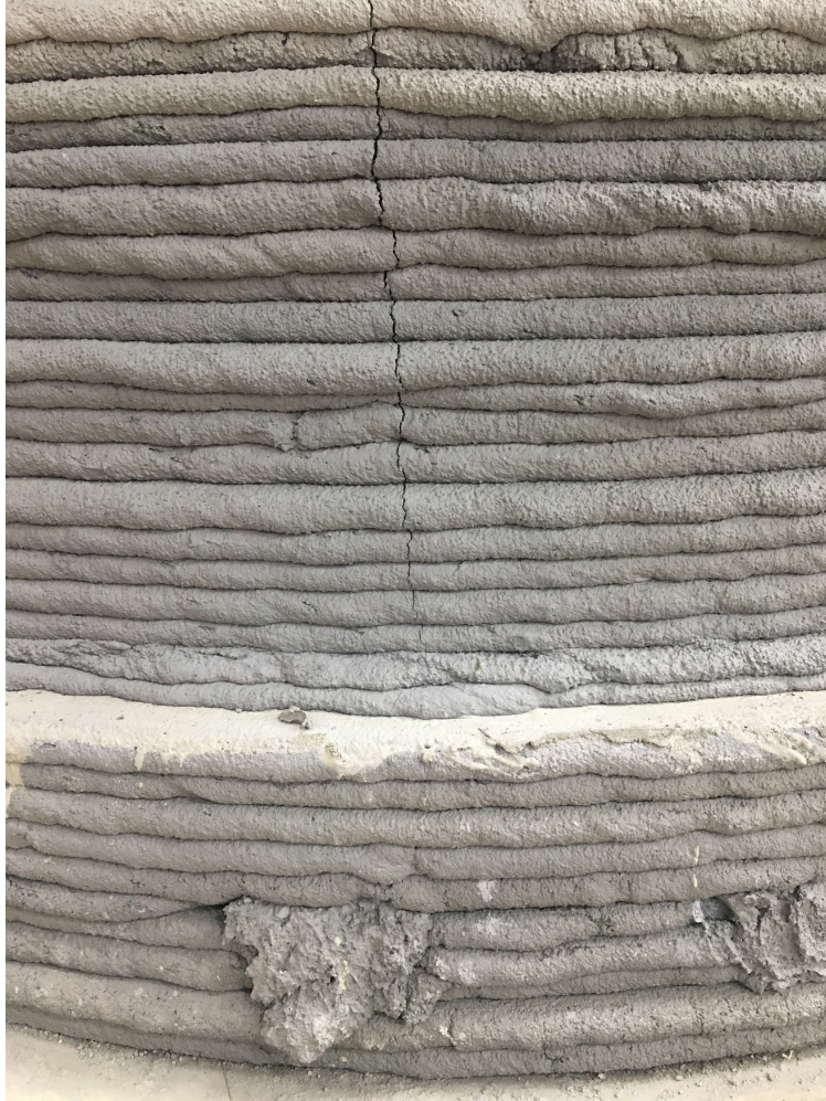
Figure 3.6: Differential shrinkage cracking in a printed part
