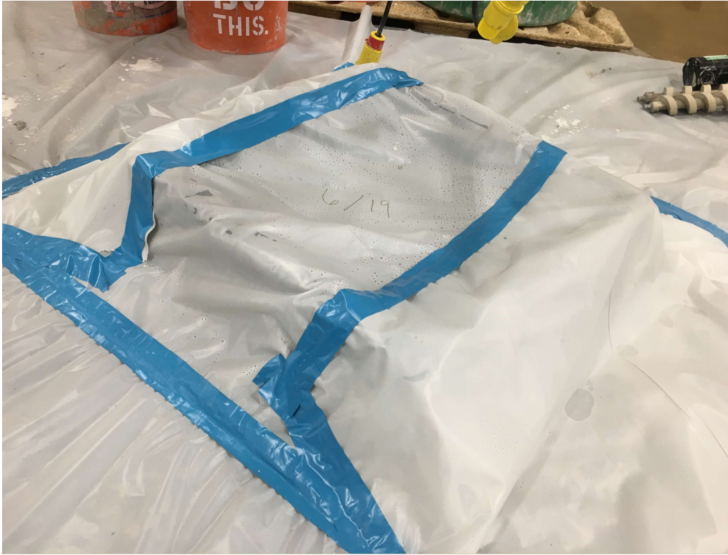
Figure 3.5: Sealed curing of the printed boxes
