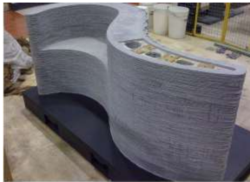
Figure 2.3: Example of Concrete Printing (from Lim et al. [8])
