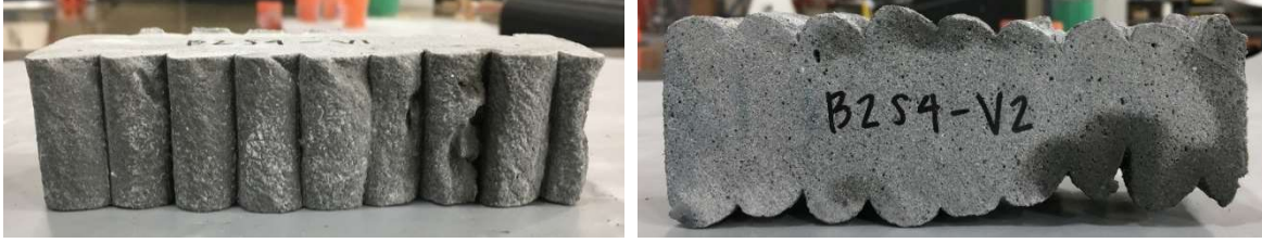
Figure 3.10: Orientations of the two different loading setups relative to the applied load and print path. Orientation A (left) and orientation B (right)
