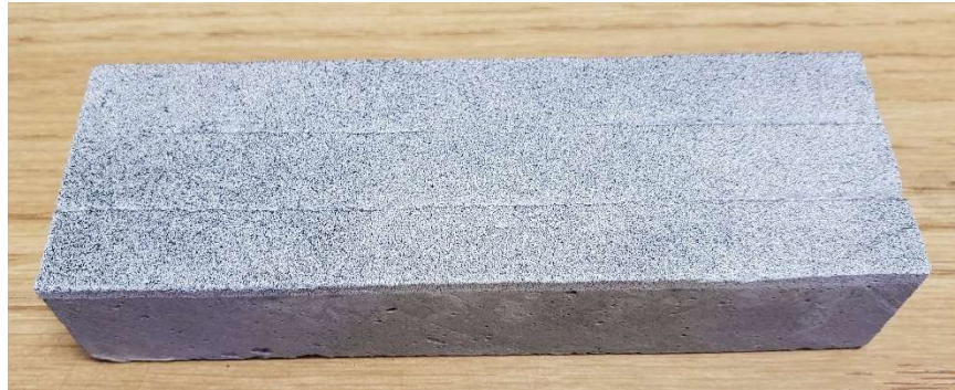
Figure 2.9: Speckle pattern applied to a beam
