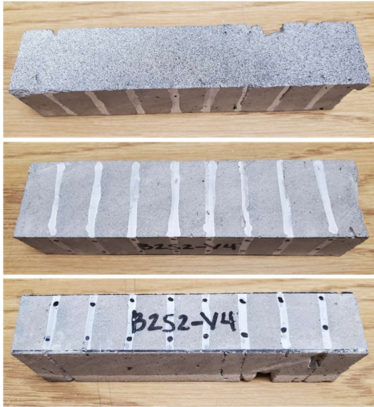
Figure C-11: B2S2-V4 prior to testing
