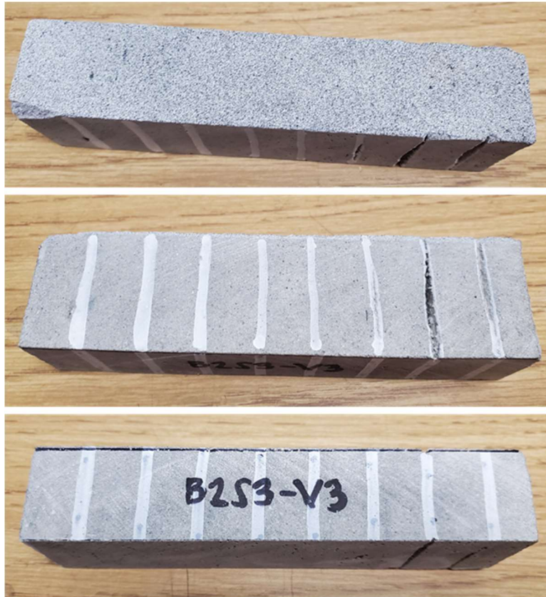
Figure C-13: B2S3-V3 prior to testing
