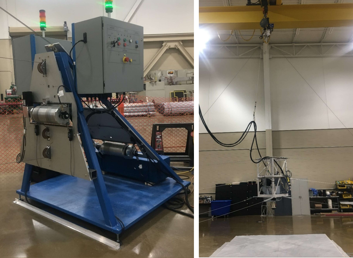
Figure 3.1: One of the SkyBAAM stations controlling xy-plane (left) and z-axis cable controlled by overhead crane (right)
