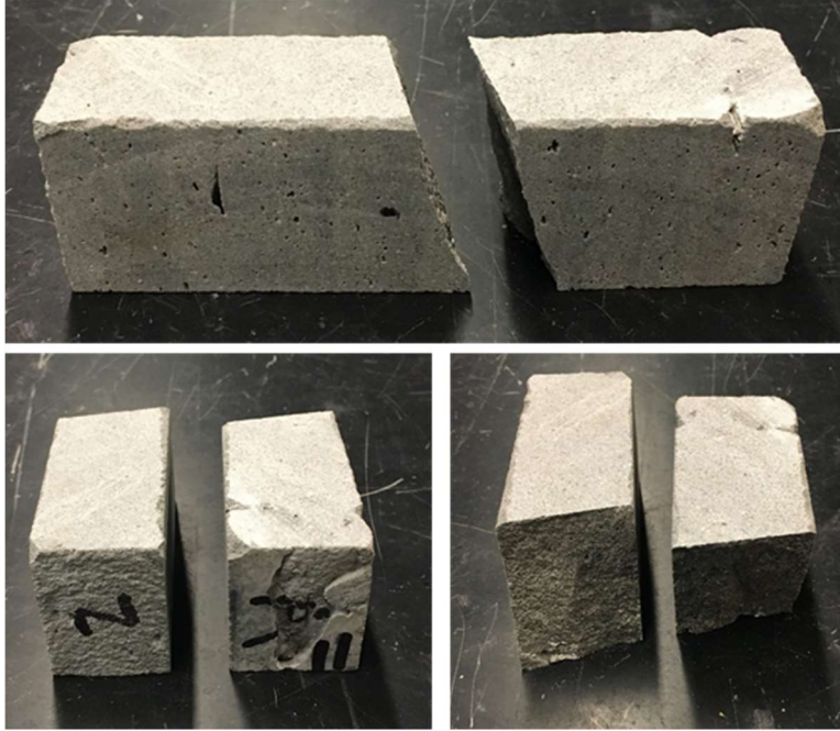
Figure A-2: BIS1-V2 after failure
