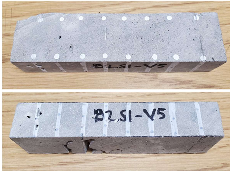
Figure C-10: B2S1-V5 prior to testing
