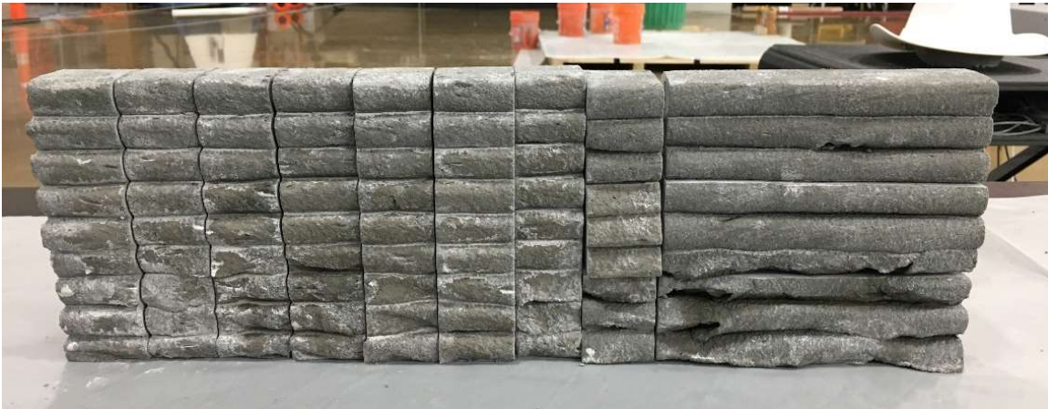
Figure 3.7: Side sawcut from printed box with the pieces all stacked in their original place
