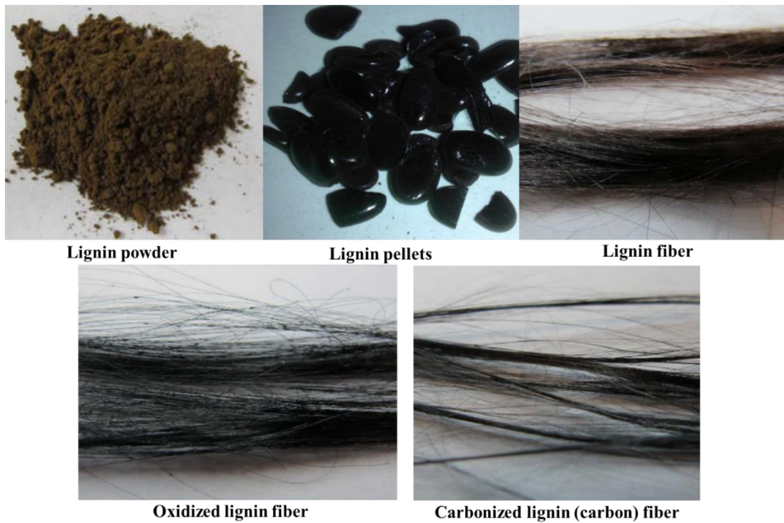
Figure 2.10 Different stages of lignin appearance from lignin precursors to form lignin-based carbon fibers. 53
