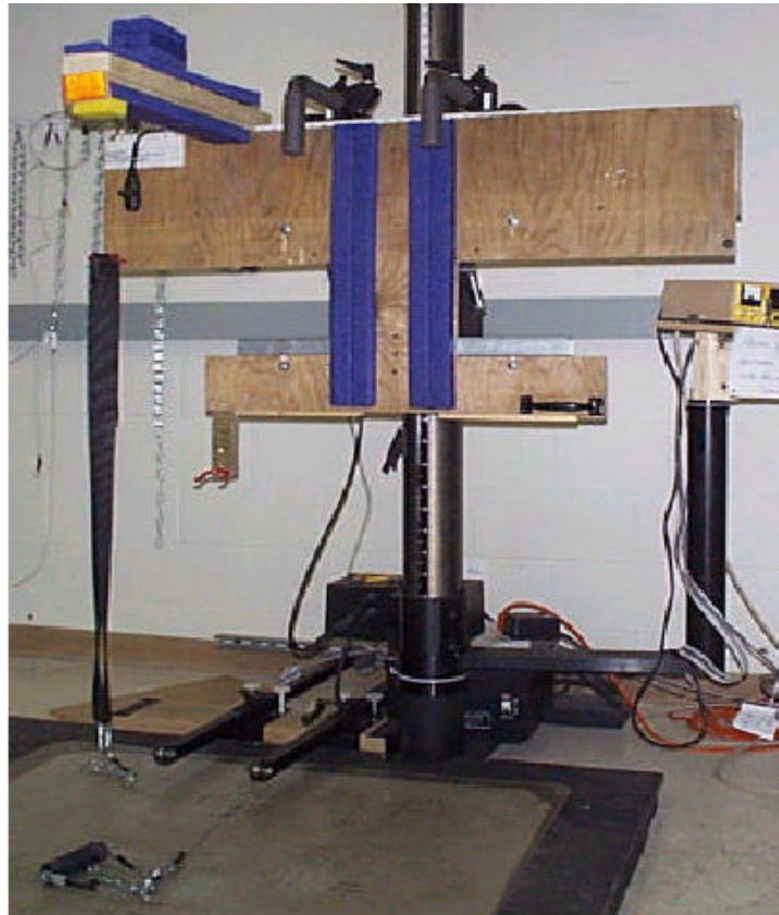
Figure 3.4. Testing fixture. The height adjustable fixture was designed to hold the shoulders against the rigid backboard. A system of straps, chains, and pulleys were used to connect handles to force transducers.
