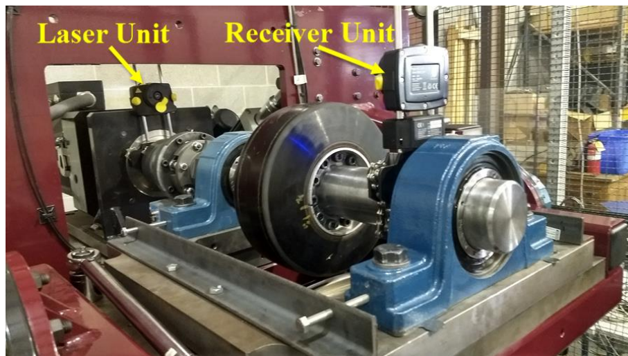
Figure 3-14 Driveline with laser sensor and receiver units mounted on either side of coupling
