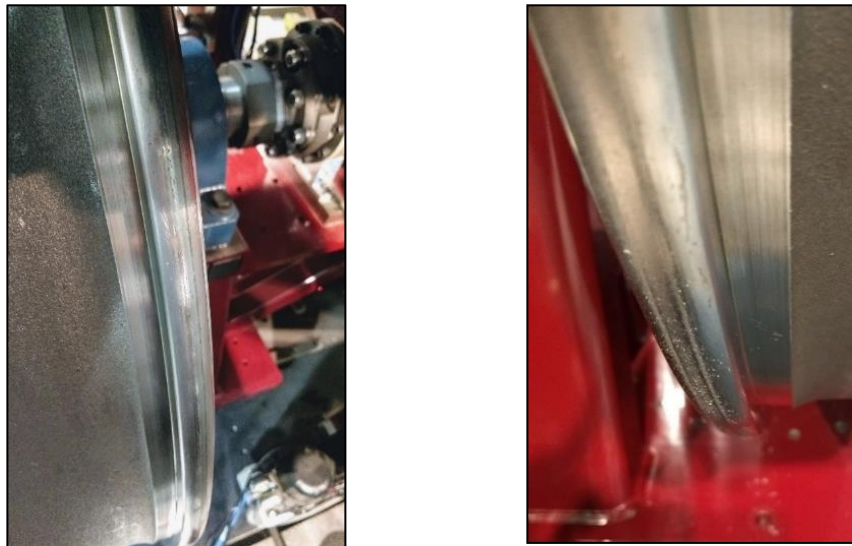
Figure 6-11 Comparison of roller profile before conducting the wear test experiment (left) and after conducting the wear test experiment (right)
