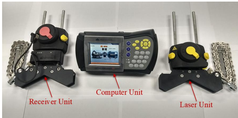
Figure 3-15 Components of the OPTALIGN smart RS5 laser alignment system
