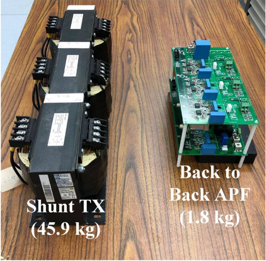
Fig. 4-30. Comparison between Y- \Delta transformer and back to back APF
