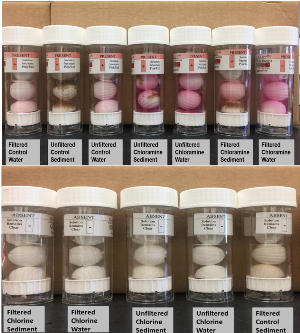
Figure 3-13 BART Nitrifier results indicated the presence of high levels of nitrifiers in the bulk water and sediment of the chloramine conditions. Development of pink color indicates the presence of nitrifiers. The intensity of the pink color is proportional to the potential nitrifiers population and is compared to a colorimetric chart to estimate the nitrifier abundance. The highest pink intensity approximates to 100,000 cfu/mL.
