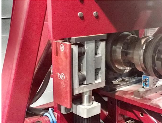
Figure 3-17: Passive rubber shear compliance on the VT-FRA Roller Rig
