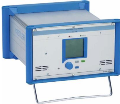
Figure 2-8: Kistler type 5070A charge amplifier used in Roller Rig force-moment measuring system
