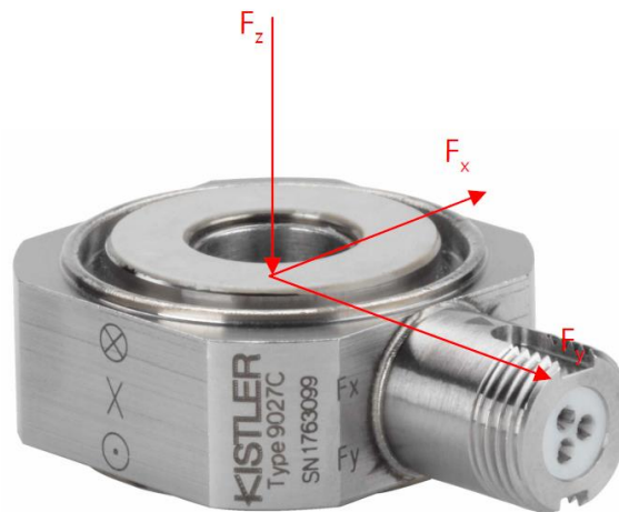
Figure 2-1 Kistler piezoelectric load cell type 9027C with load directions shown [2]
