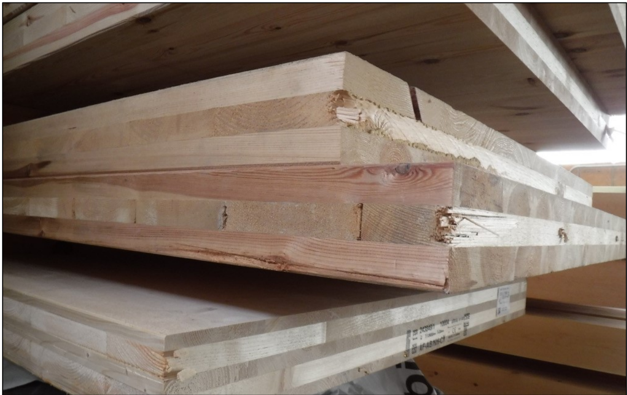
Figure 2: Example photo of CLTs taken at Sauter Timber (A.L. Hammett, 2019).
