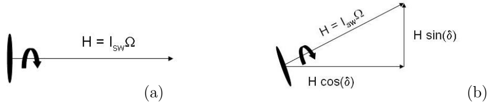
Figure 6.2: Change in Angular Momentum from Gimbaling
