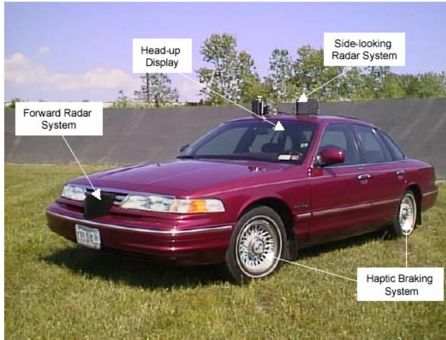
Figure 2.7 - The ICAS Test-Bed
