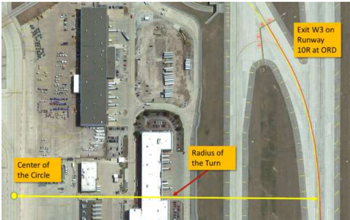
Figure 3 : Radius of the Turn for a High-Speed Exit W3 on Runway 10R at ORD.
