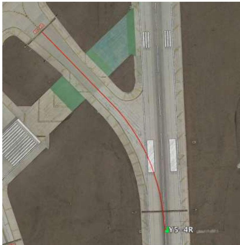
Figure 30 : Exit Y5 on Runway 4R at ORD Having Large Hold Bar Distance.
