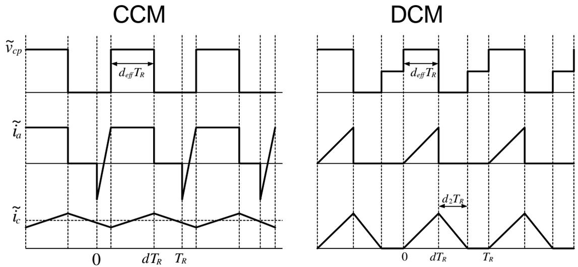
**Figure 2.6.** Averaged Switch Model terminal quantities for FB-PWM converter
