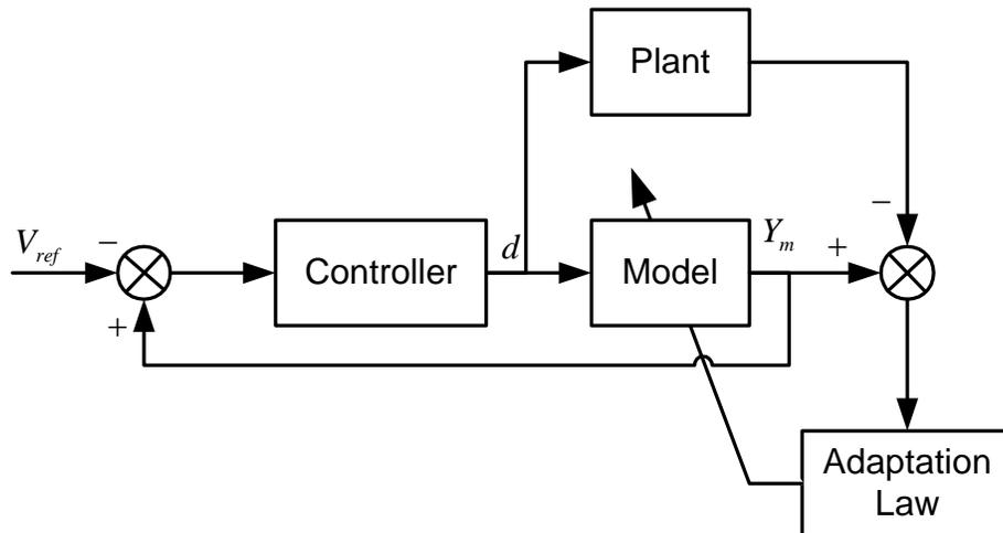
**Figure 1.9.** Basic configuration of an adaptive model
