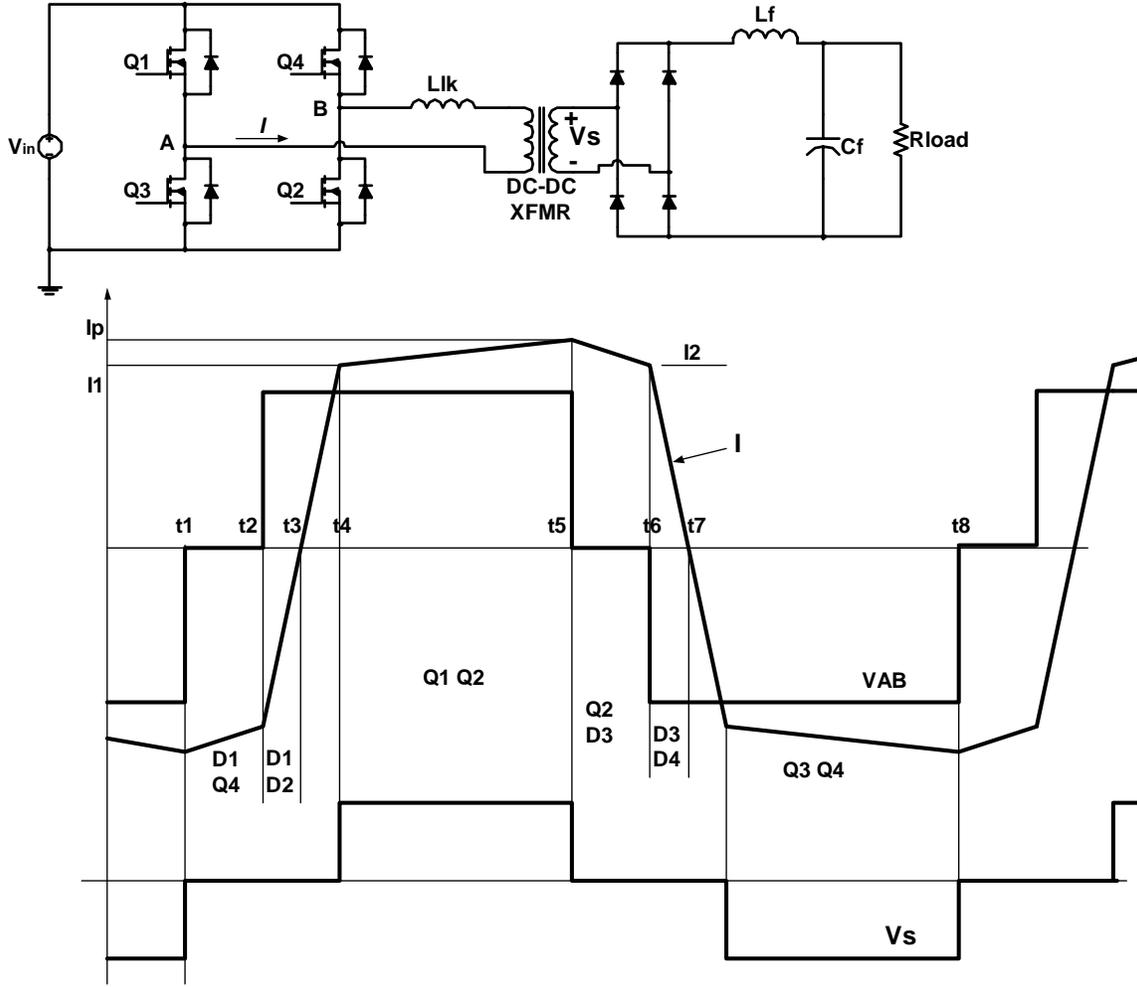
Figure 2.3. Principle of Operation of Phase Shifted FB-PWM Converter
