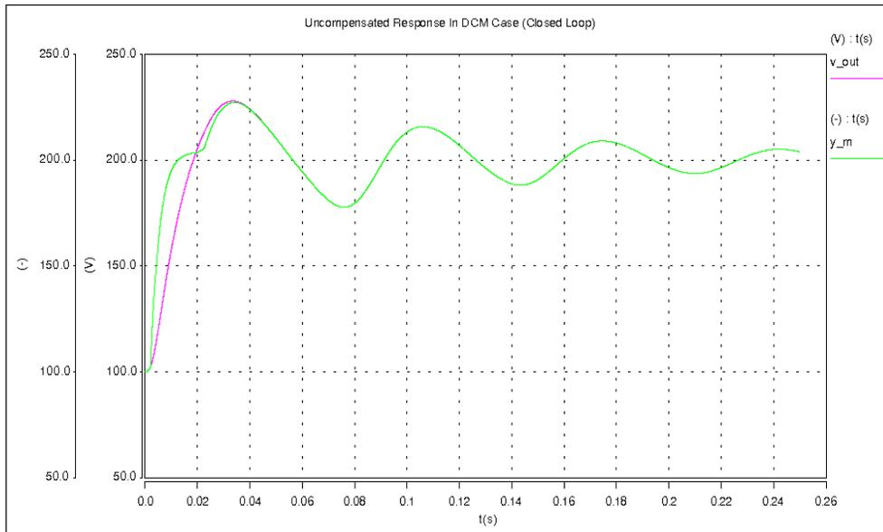
**Figure 3.7.** Closed loop performance with a PI controller.
