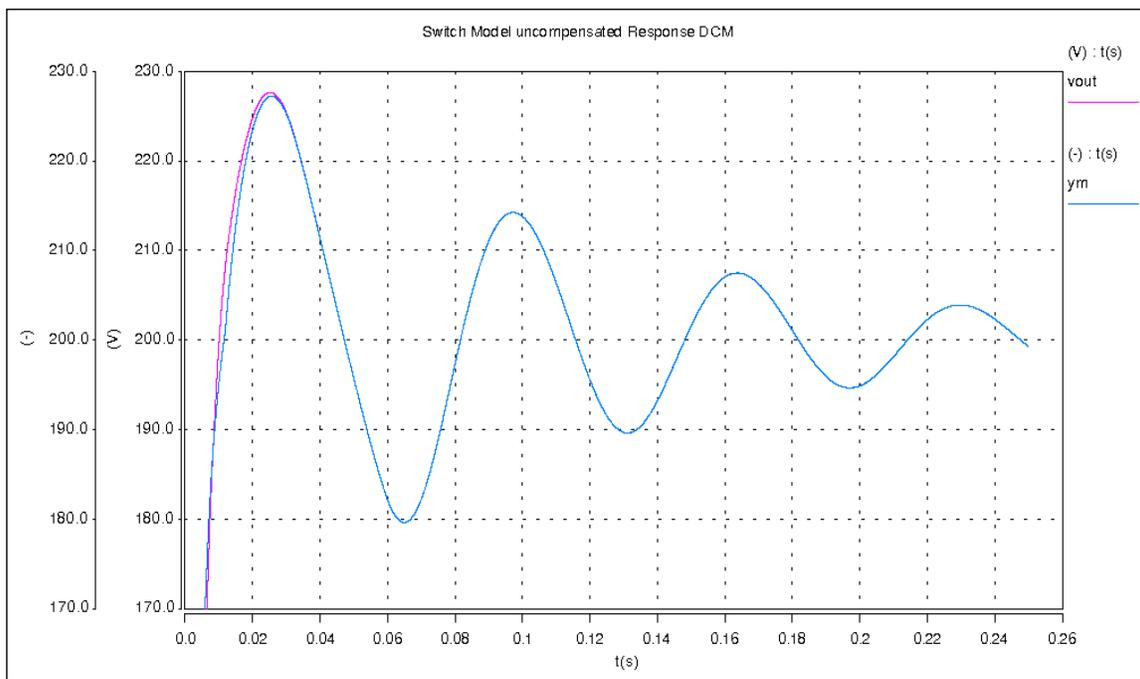
**Figure 3.15.** Switch model with only PI controller
