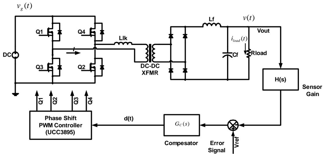
Figure 1.3. Voltage Mode Control
