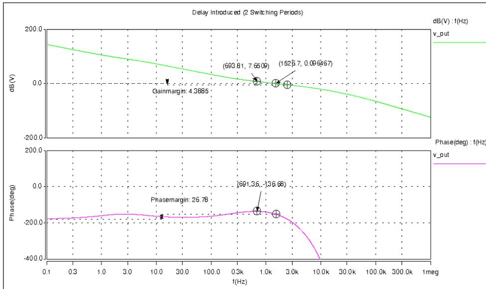
**Figure 3.11.** Frequency response after delay is added.
