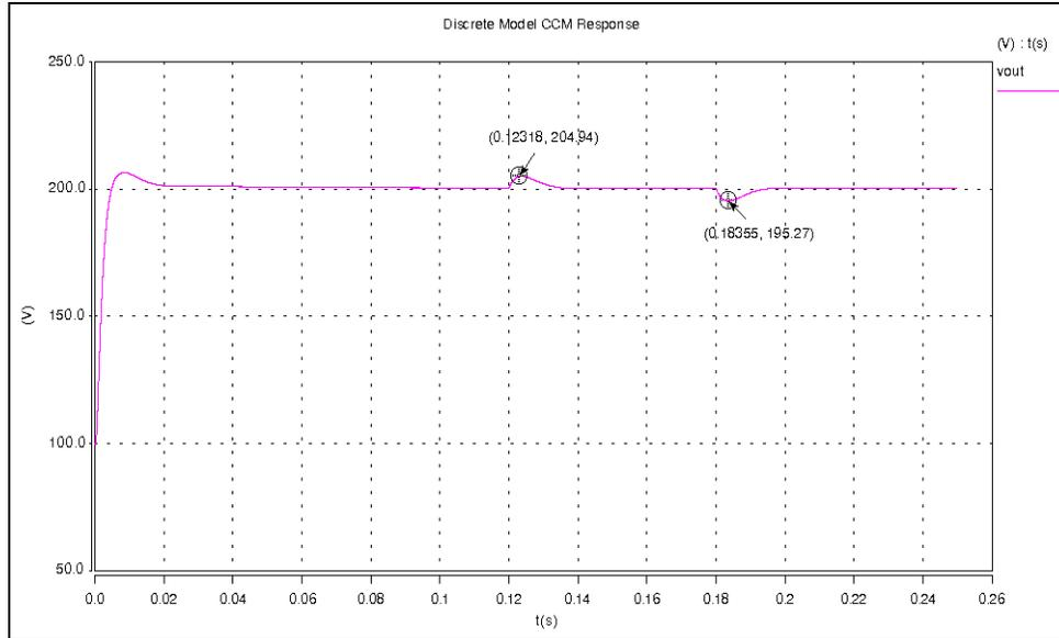
**Figure 3.17.** 50% load step in CCM model
