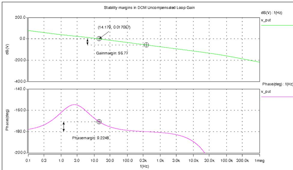
**Figure 3.8.** Loop Gain Frequency response with simple PI controller.
