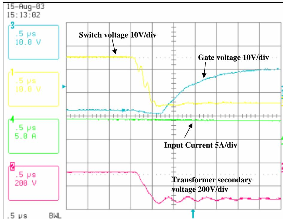
Figure 4.14. Switching Waveforms
