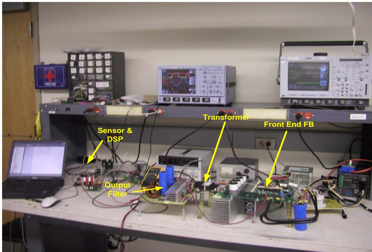
Figure 4.13. Bench Test Set-Up
