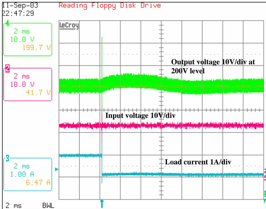
Figure 4.23. 50 % load decrease input voltage at 22V
