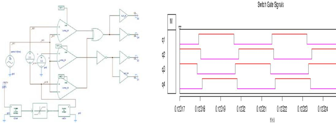
**Figure 3.14.** Implementation of the UCC3895 and its Corresponding Switch Waveforms.
