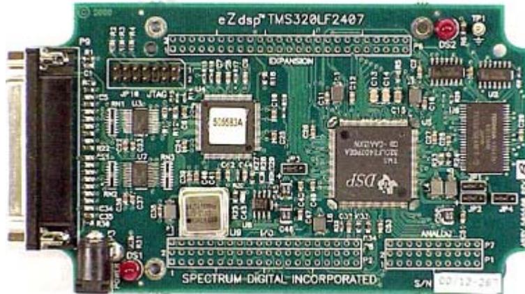
**Figure 4.7.** Texas Instruments TMS320LF2407A DSP.
