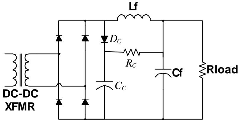
Figure 4.17. Passive Clamp Design
