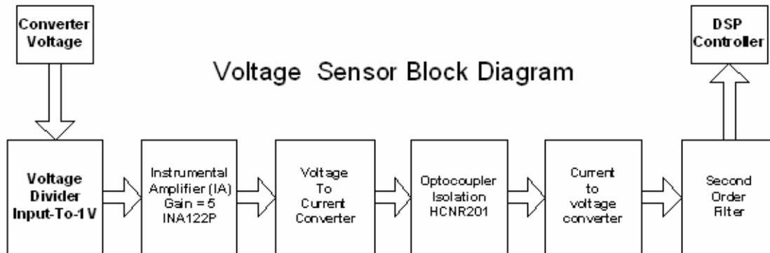
Figure 4.2. DC Sensor Block Diagram
