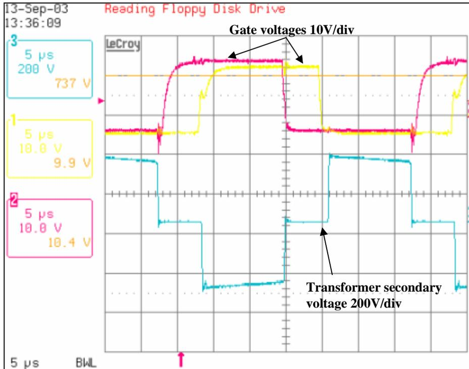
Figure 4.15. Phase Shifting Operation.
