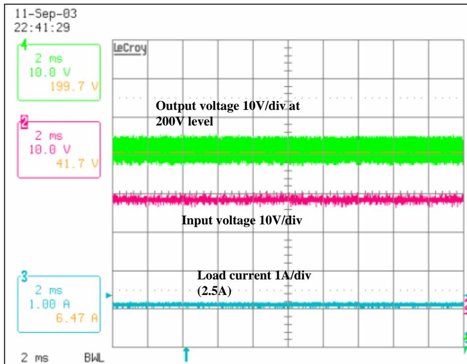
Figure 4.19. Steady State input voltage 28V output voltage 200V
