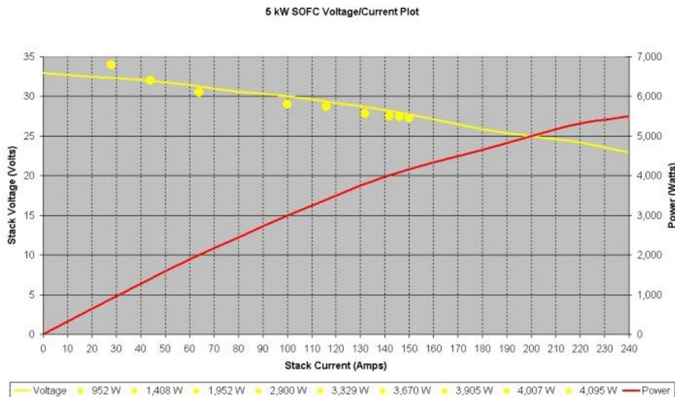
**Figure 1.2.** Voltage to current plot of a solid oxide fuel cell (SOFC)
