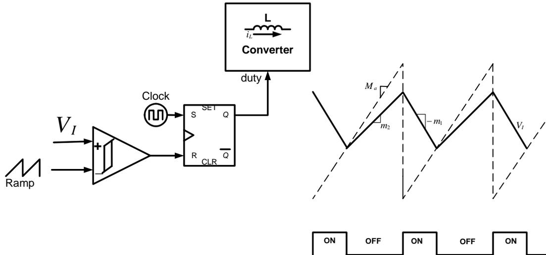
Figure 1.8. Sensorless Current Mode Control
