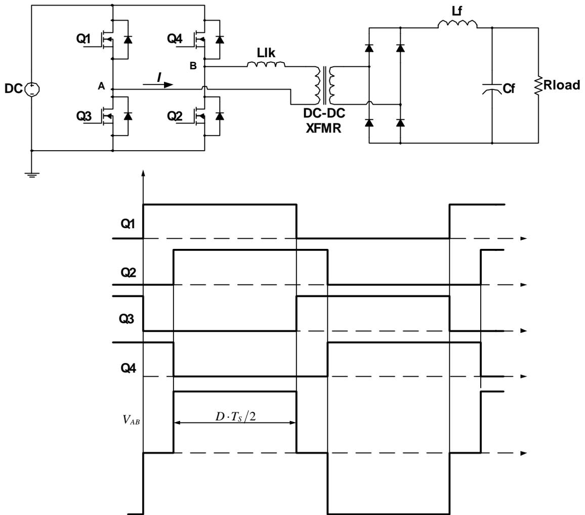
Figure 2.2. Phase Shifted FB-PWM Converter
