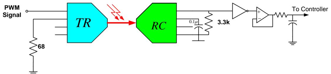
**Figure 4.8.** Optical isolation circuit for PWM transmission
