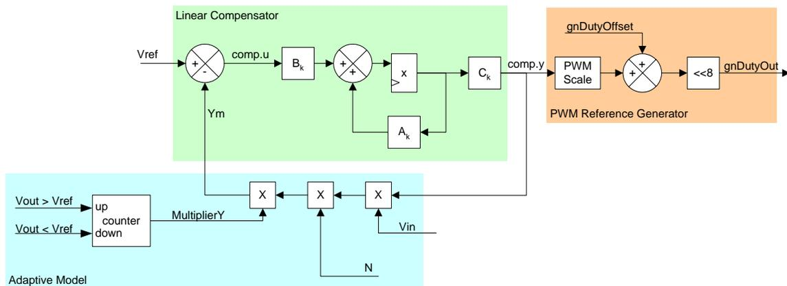
**Figure 4.12.** Control Algorithm Description
