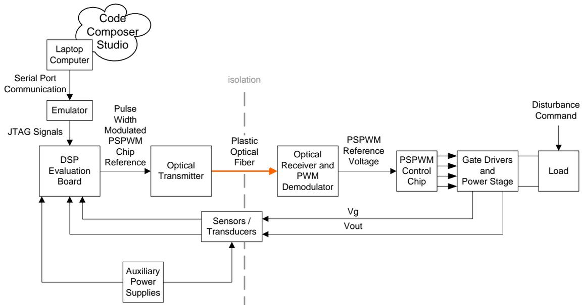
**Figure 4.9.** Control System Configuration
