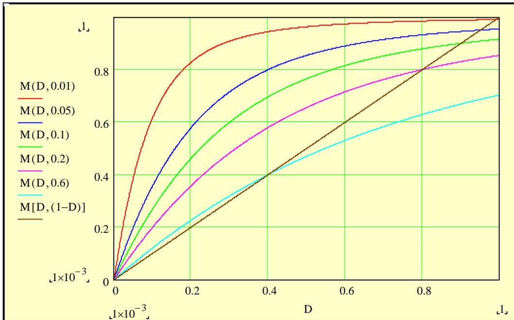
**Figure 2.5.** Modulation index vs. Duty cycle
