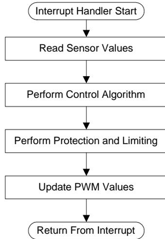
**Figure 4.10.** Interrupt Handler Flow Chart
