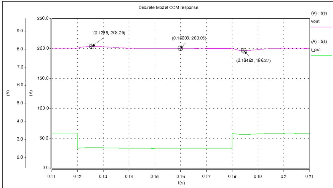
**Figure 4.25.** Simulation Load steps from 750W to 500W and from 500W to 750W
