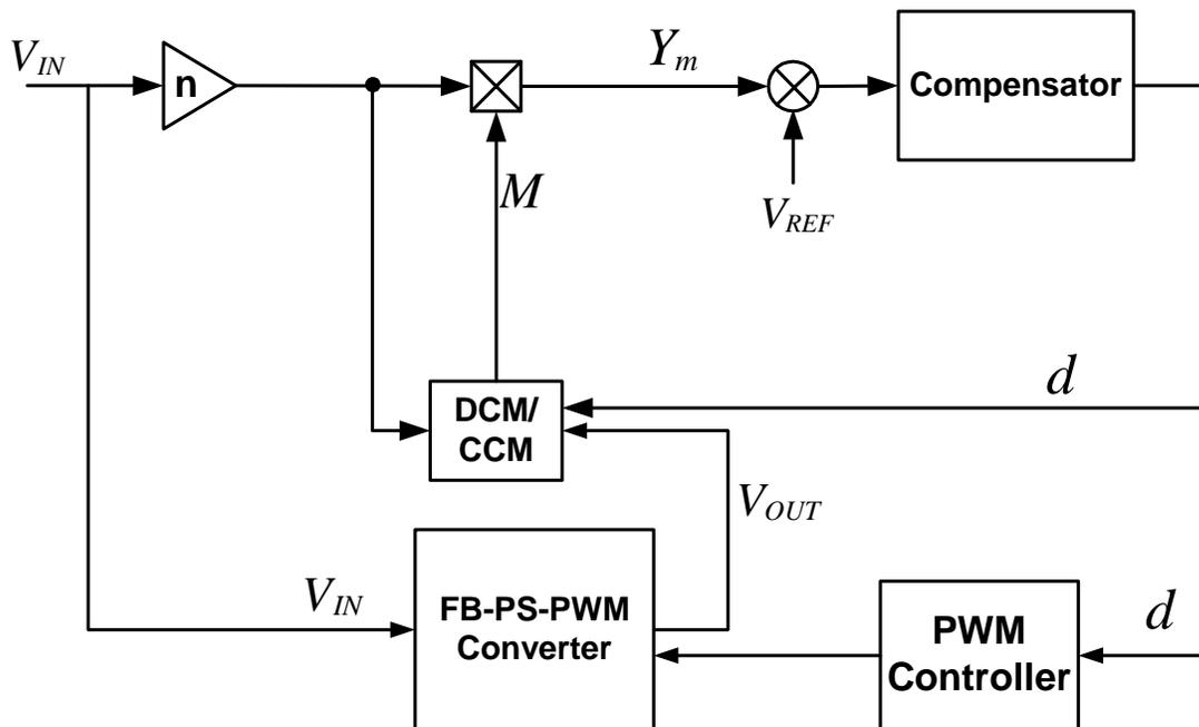
Figure 3.1. Block Diagram Model Reference Controller
