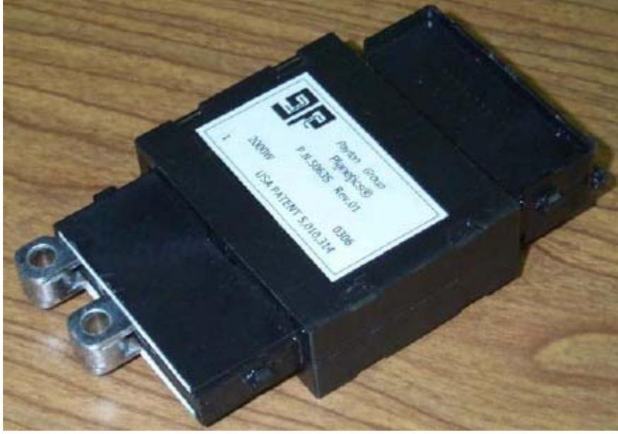
Figure 4.5. 2kW planar transformer
