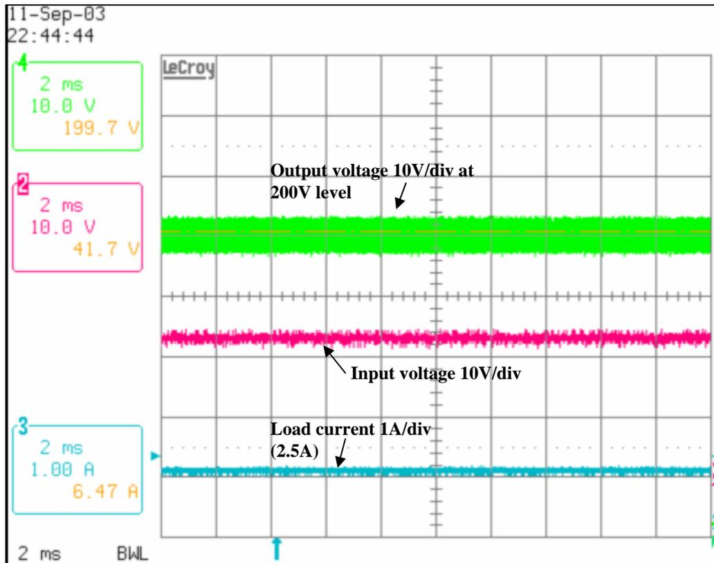
**Figure 4.20.** Input reduced to 22V and output at 200V
