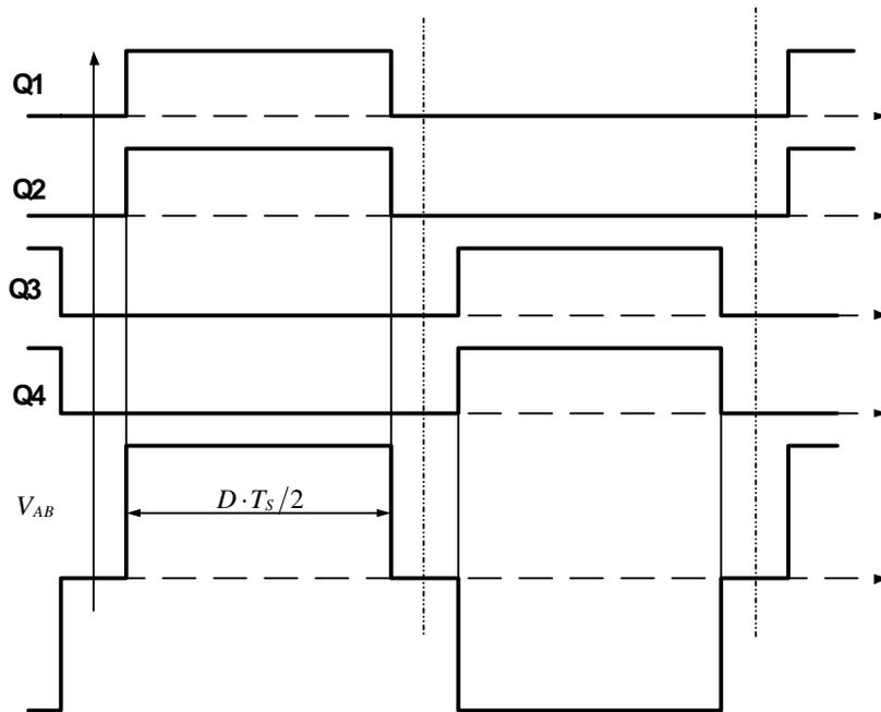
**Figure 2.1.** Conventional FB-PWM Converter
