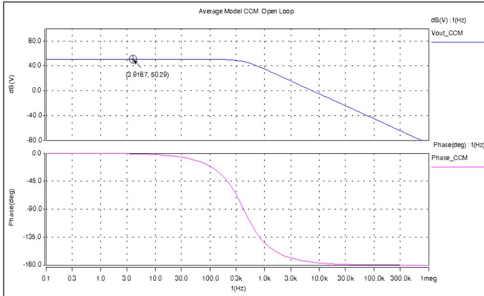
**Figure 3.4.** Control-to-output transfer function in CCM.
