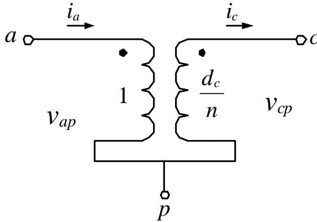
**Figure 2.7.** Three-terminal averaged ZVS PWM Switch Model
