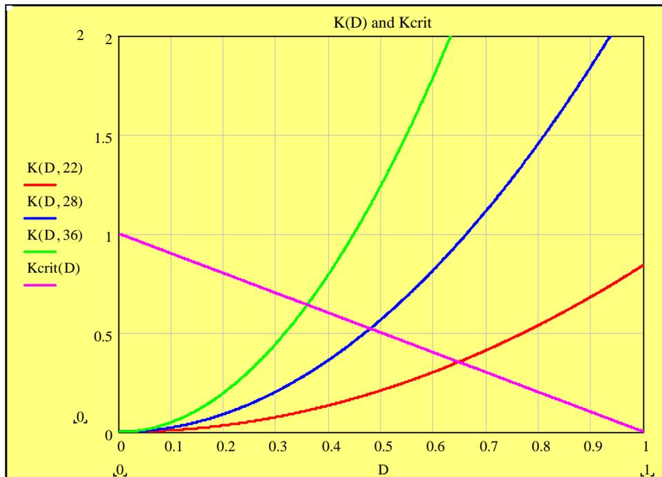
**Figure 2.4.** Coefficient k as a function of Duty Cycle
