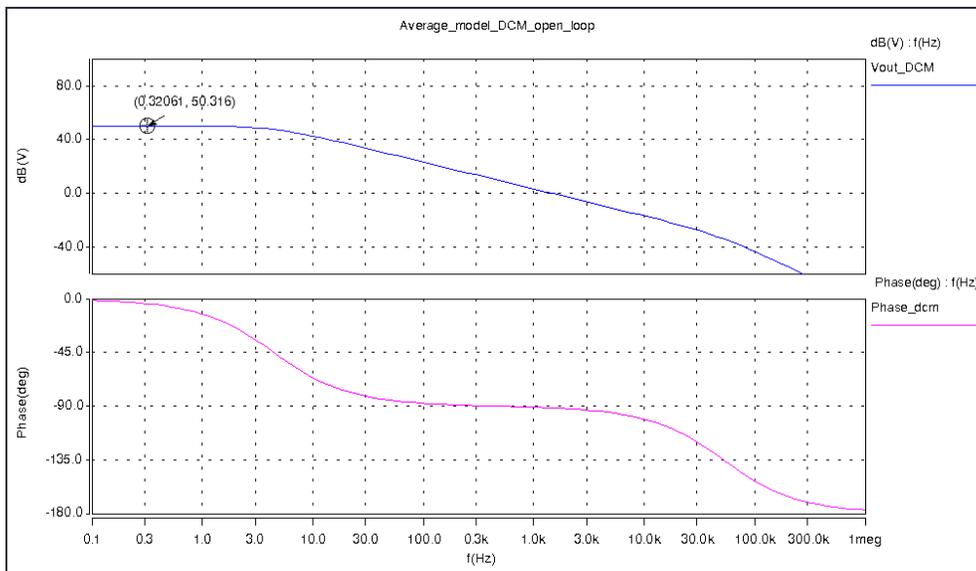
**Figure 3.5.** Control-to-output transfer function for DCM operation.
