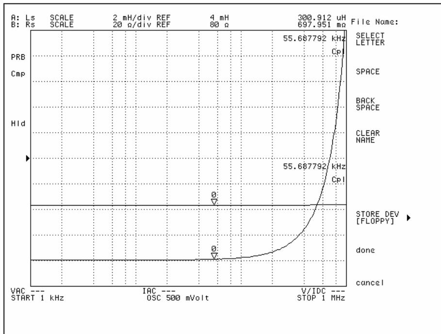
**Figure 4.6.** Measured Inductor Value
