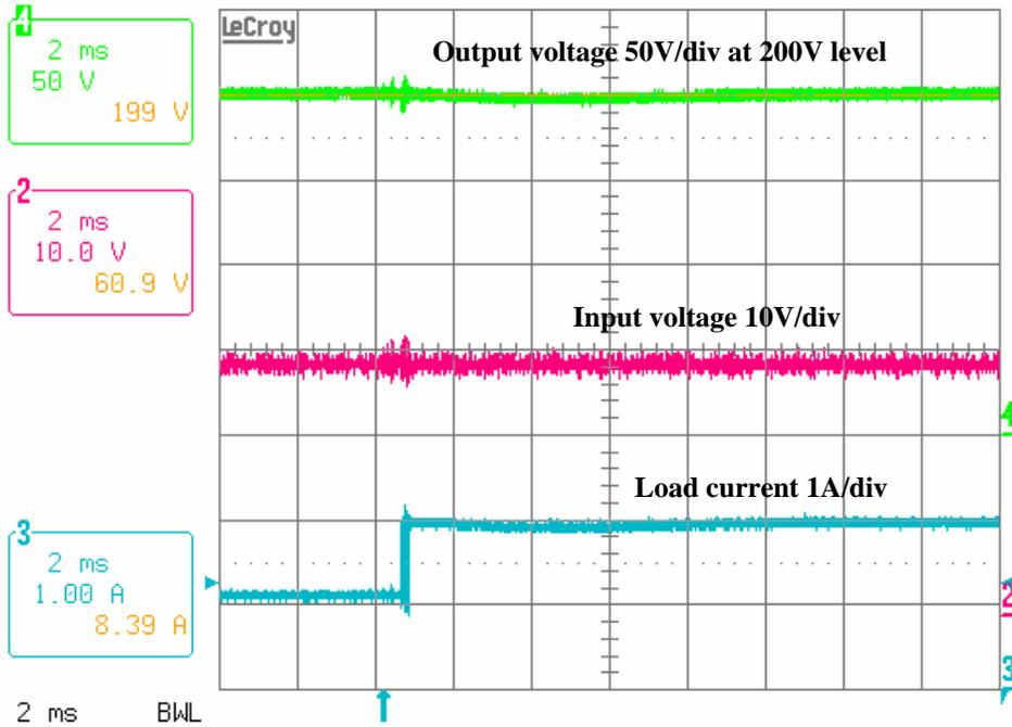
Figure 4.26. Load increase from 500W to 700 W
