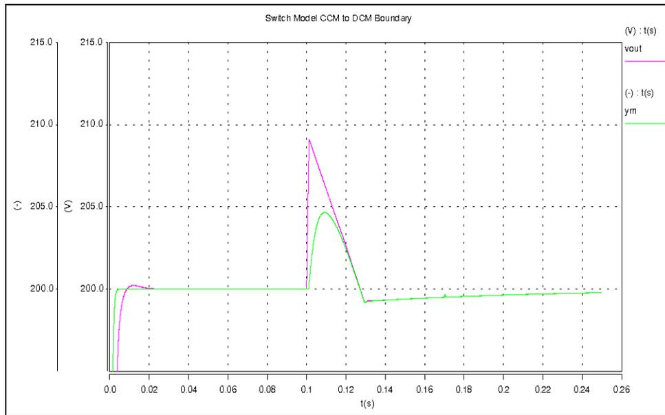
**Figure 3.16.** Boundary between CCM and DCM operation
