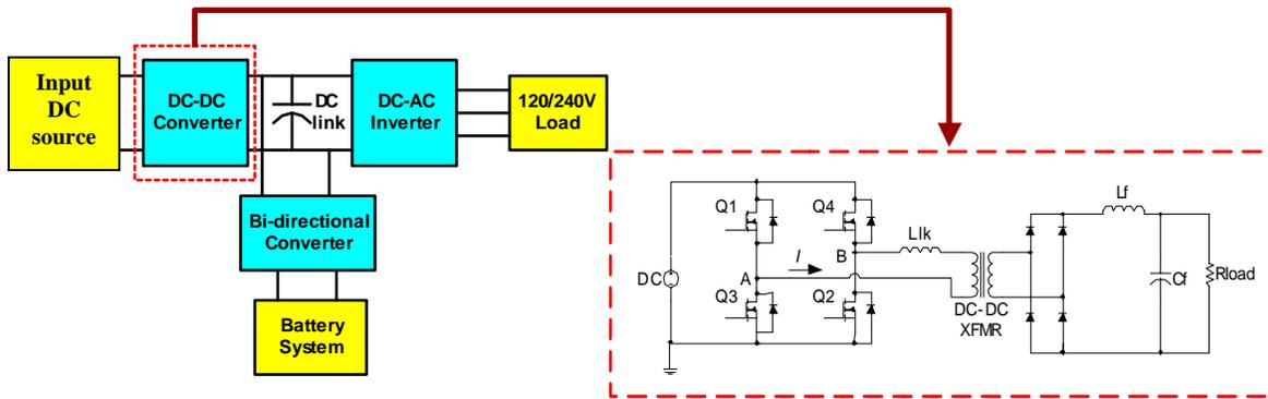
**Figure 1.1.** Basic block diagram of the power conversion system
