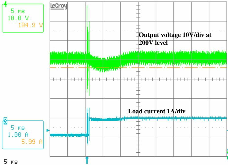
Figure 4.21. Load increase from 500W to 750W
