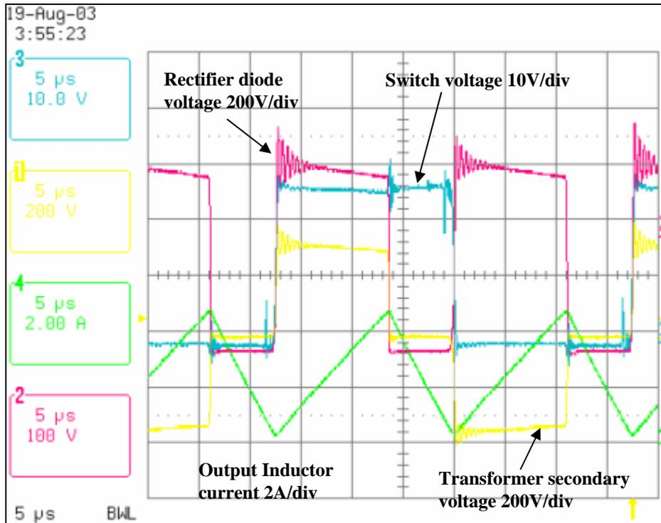
Figure 4.16. Output Waveform and diode ringing
