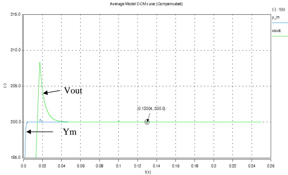
**Figure 3.10.** Transient performance with the improved controller
