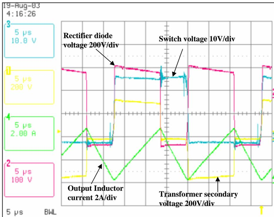
Figure 4.18. Output Waveform After Clamp is Included in the Circuit
