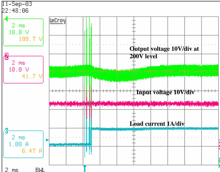
Figure 4.24. 50% load increase at 22V input.
