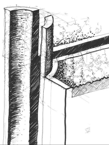
the water passes through a concrete "half-pipe" down to the cabin below
