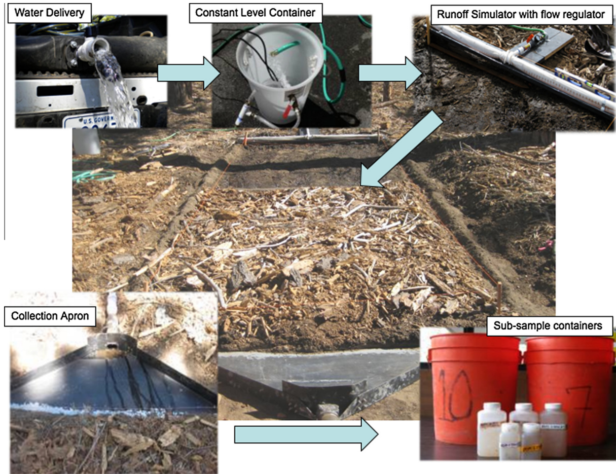
Fig. 5. Flow chart depicting snowmelt runoff simulation methodology. Water was applied evenly at the top of a 10 m 2 plot. Runoff was collected at the bottom of the plot, allowing for the measurement and observation of rill erosion processes at a scale applicable to hillslope erosion.
