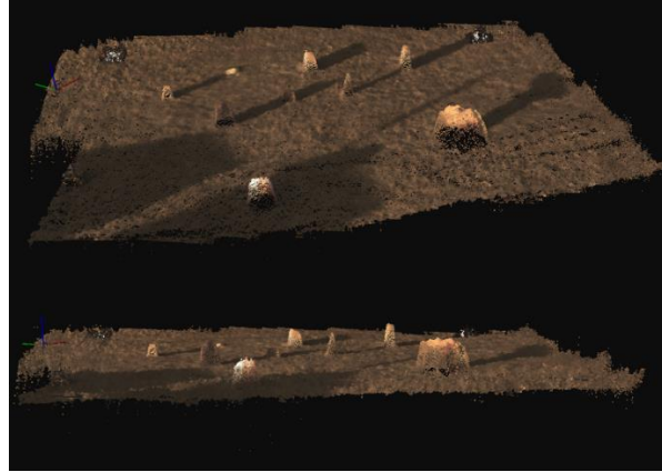
Figure 21: Point cloud created with voxel size 2.5 cm; points 343,511, file size 5.2 Mb
