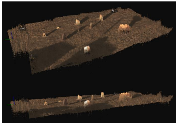
Figure 20: Point cloud created with voxel size 1 cm; points 2,129,850, file size 32 Mb
