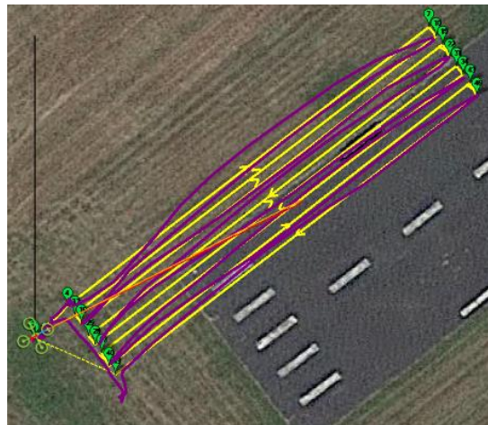
Figure 12: Lawn mower path pattern of UAV for image collection
