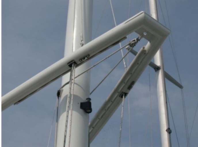
Figure 101- Wishbone Boom Attached to Mast
