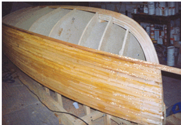
Figure 65- Strip Planking Construction (Selway Fisher Design, 2009)
