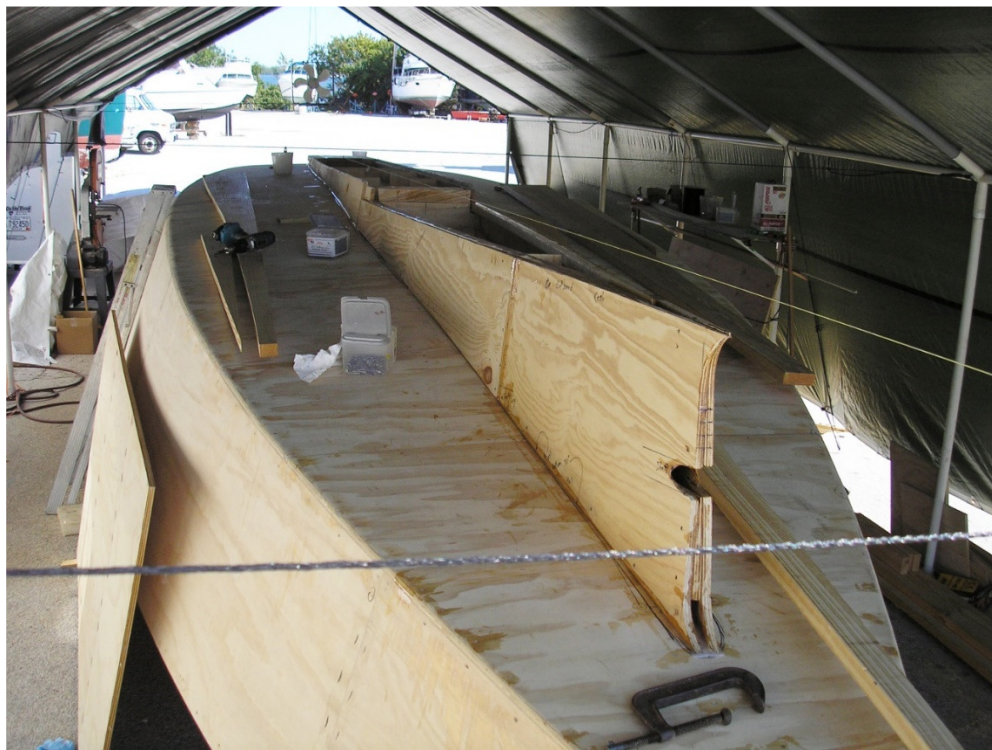
Figure 64- Sharpie Cold Molded Construction Plywood/Epoxy
