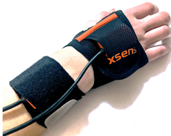
Figure 3.3: A pair of Xsens inertial sensors attached to the hand and wrist. The glove contains a pouch with velcro for attaching an inertial sensor and webbing that constrains the sensor from rotating. The wrist's inertial sensor was attached to a portion of the strap and then wrapped with the remainder of the strap to constrain it further and avoid any additional rotation.
