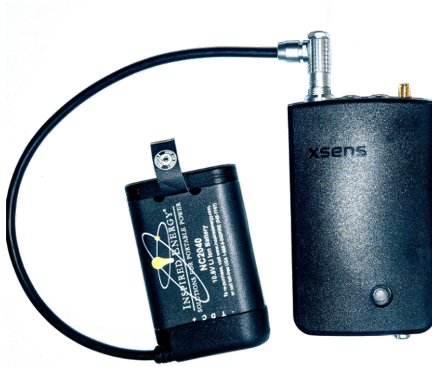
Figure 3.2: A bodypack connected to a battery. The bodypack also has two ports for connecting the sensors. The button on the lower right of the bodypack is for turning on/off the bodypack, and for starting a calibration or data collection session.
