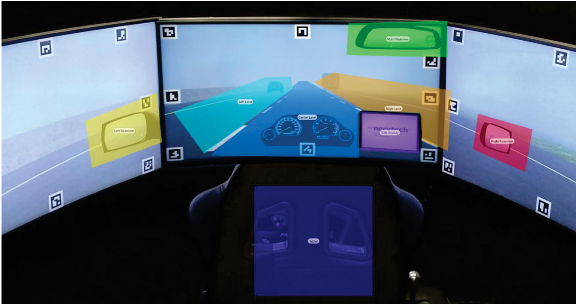
Figure 24: Areas of Interest: Side View Mirrors, Rearview Mirrors, Current Lane (Middle), Changing Lane (Right or Left Lane), Tablet and TOR Display
