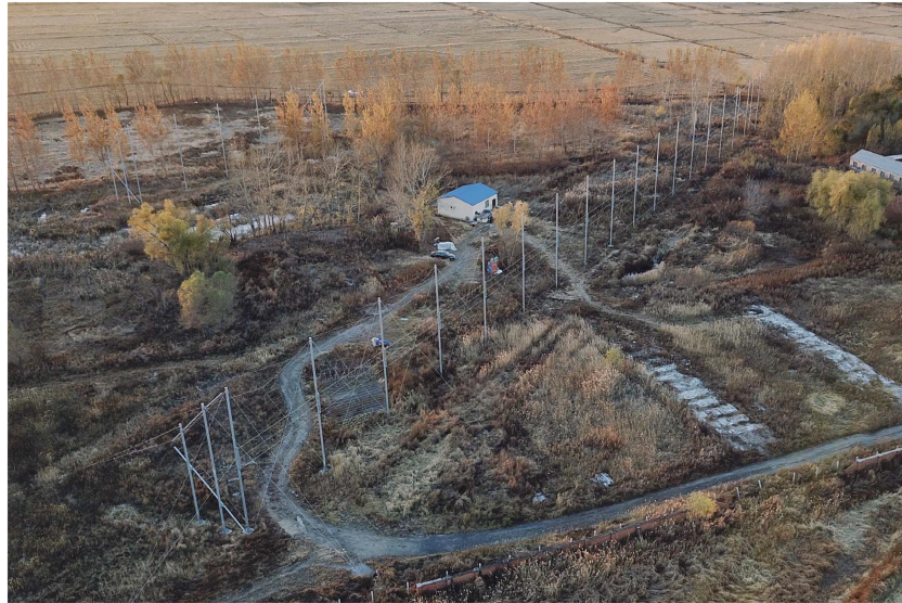
Figure 1. A bird's eye view of the Jiamusi radar site taken by a small unmanned aerial vehicle with the main antenna array across the picture from the bottom left to the top right, the interferometric array pictured in the upper left, and the equipment shelter with the blue roof located between the two antenna arrays.
