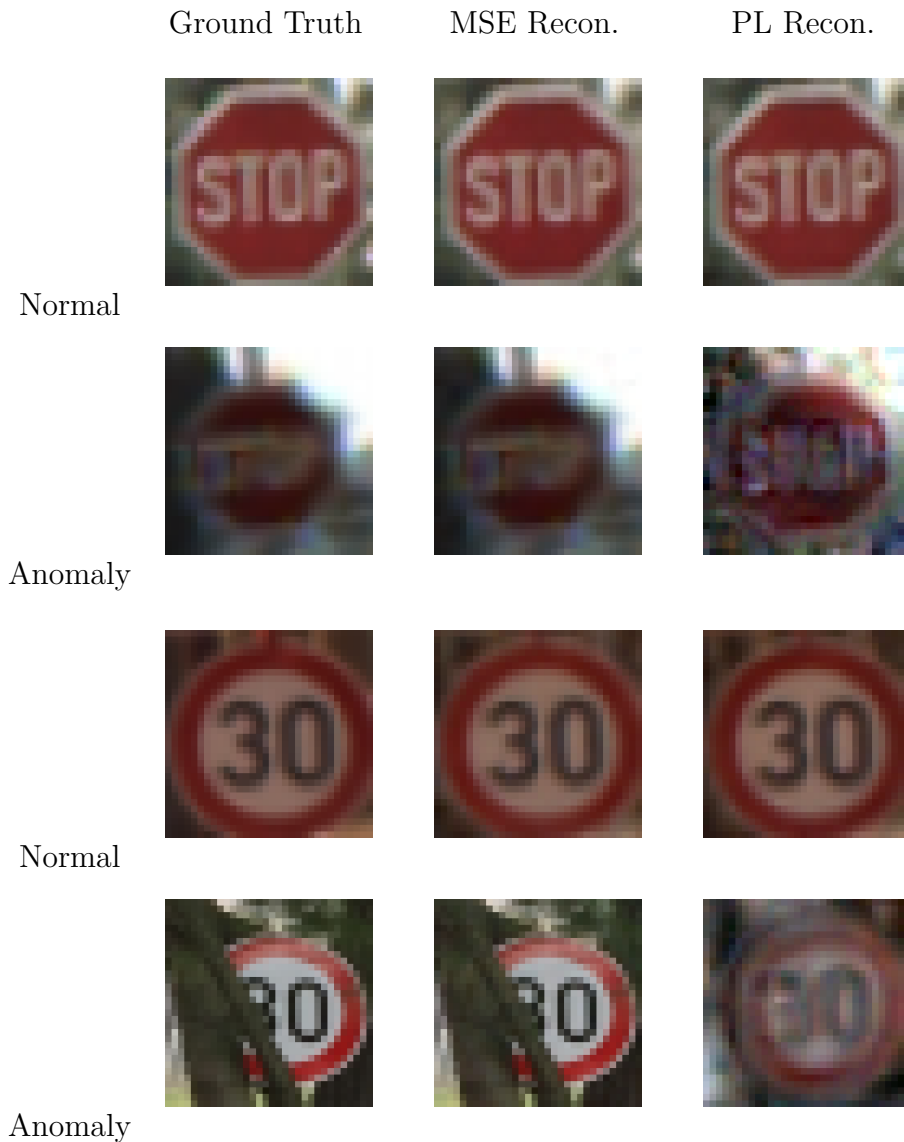
Figure 5.7: After only 50 epochs the anomaly is reconstructed under the standard MSE objective. With PL, the AE does not reconstruct the anomalous example.
