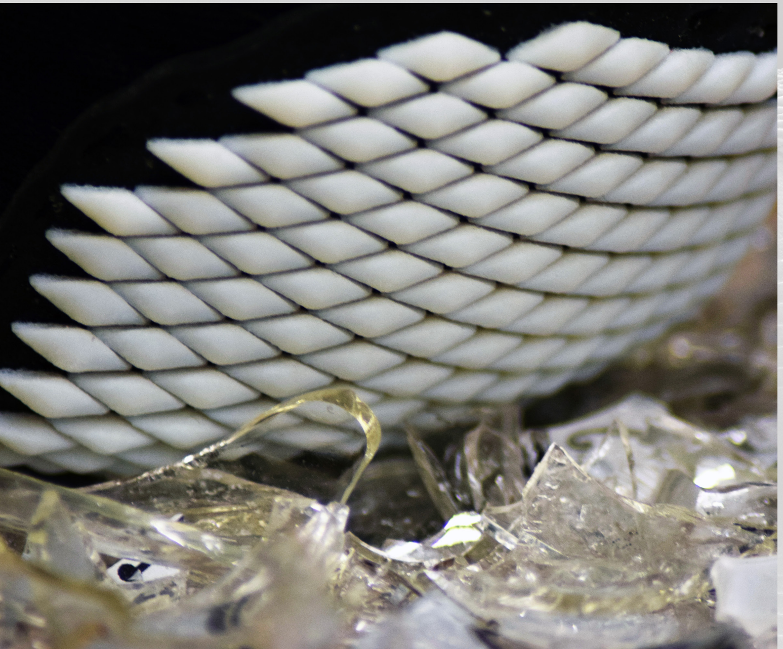
Above: The flexible armor tested on a bed of broken glass. Right: The armor is printed with multi material 3D printing allowing for strong scales to be embedded in a flexible base. Far right top: The flexibility of the armor on display on a roller. Far right middle: a microscopic close-up view of chiton scales from the side. Far right, bottom: A chiton mollusk - the creatures measure about 1 inch in length.
