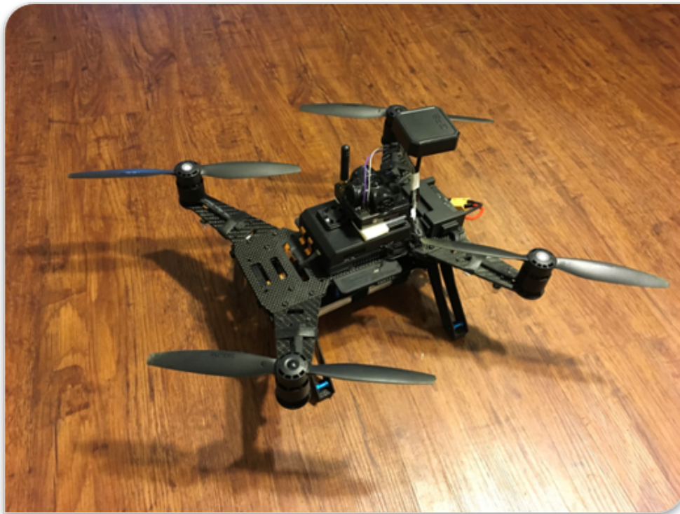
Figure 4.7: Intel Aero drone with GPS unit mounted on the top
