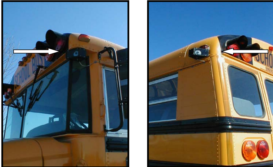
Figure 9. Violation detection cameras on front and rear of school bus.
