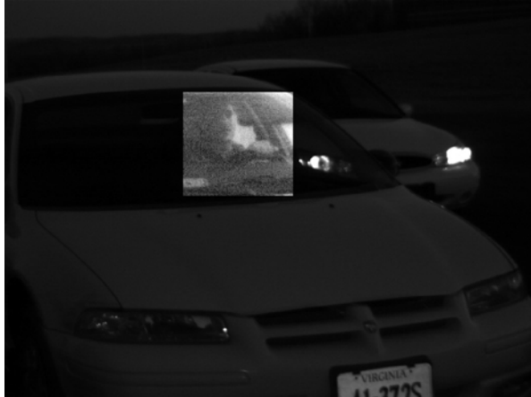
Figure 48. No headlight interference (left) and headlight interference (right). Headlight interference from the violating vehicle and/or other vehicles can degrade facial image quality, but has no noticeable impact on license plate image quality. Violating vehicle is traveling approximately 15 mph and the secondary vehicle is stationary.
