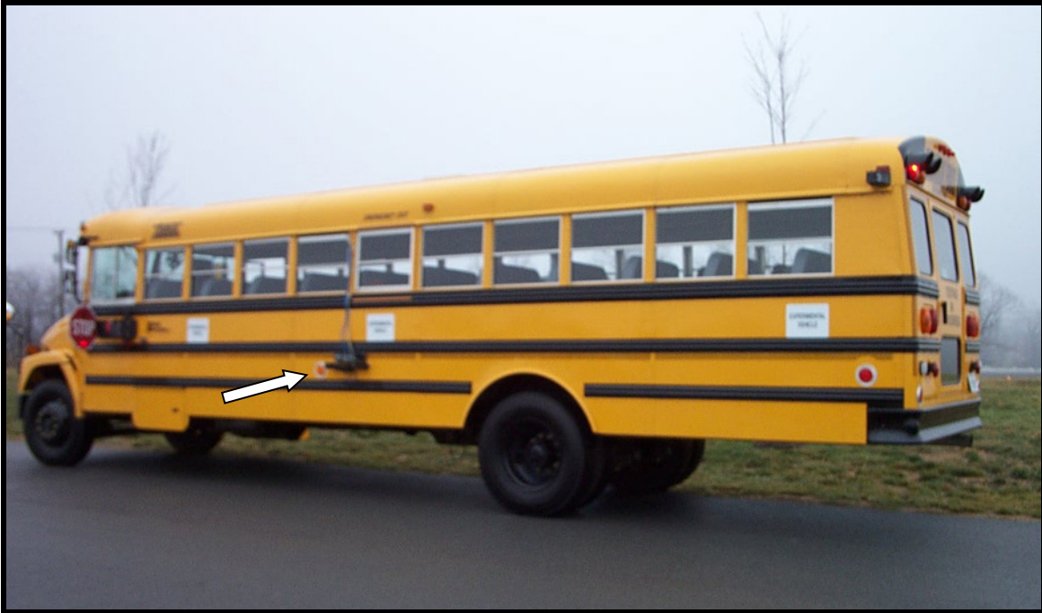
Figure E-2. Violation recording cameras positioned in a central location.
