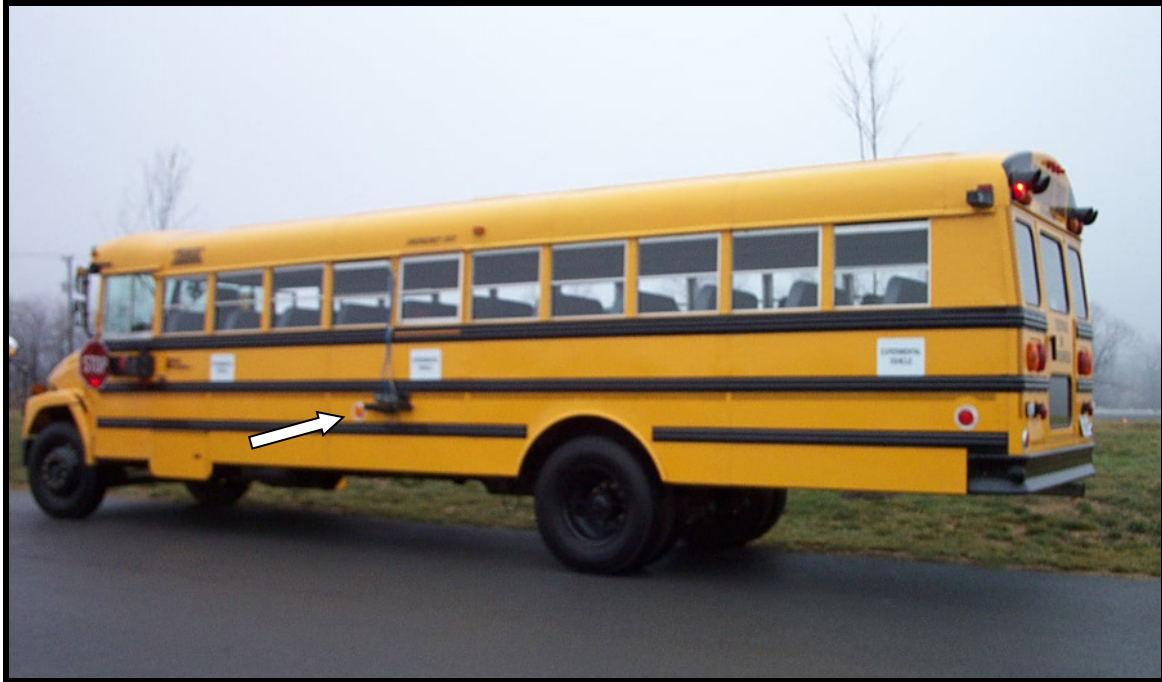
Figure 10. Violation-recording cameras positioned in a central location.
