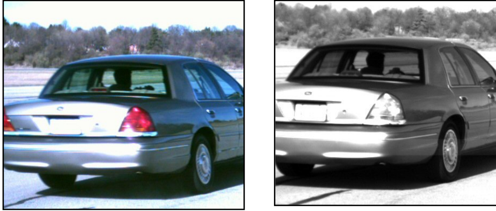
Figure 45. License plate washed out from sun; color and monochrome cameras.
