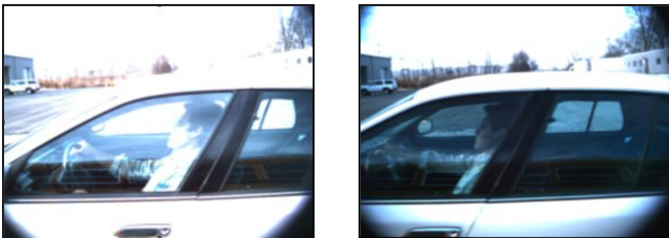
Figure 46. Facial image quality improved with the use of polarized lenses.
