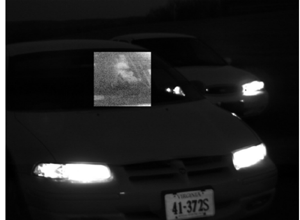
Figure 48. No headlight interference (left) and headlight interference (right). Headlight interference from the violating vehicle and/or other vehicles can degrade facial image quality, but has no noticeable impact on license plate image quality. Violating vehicle is traveling approximately 15 mph and the secondary vehicle is stationary.
