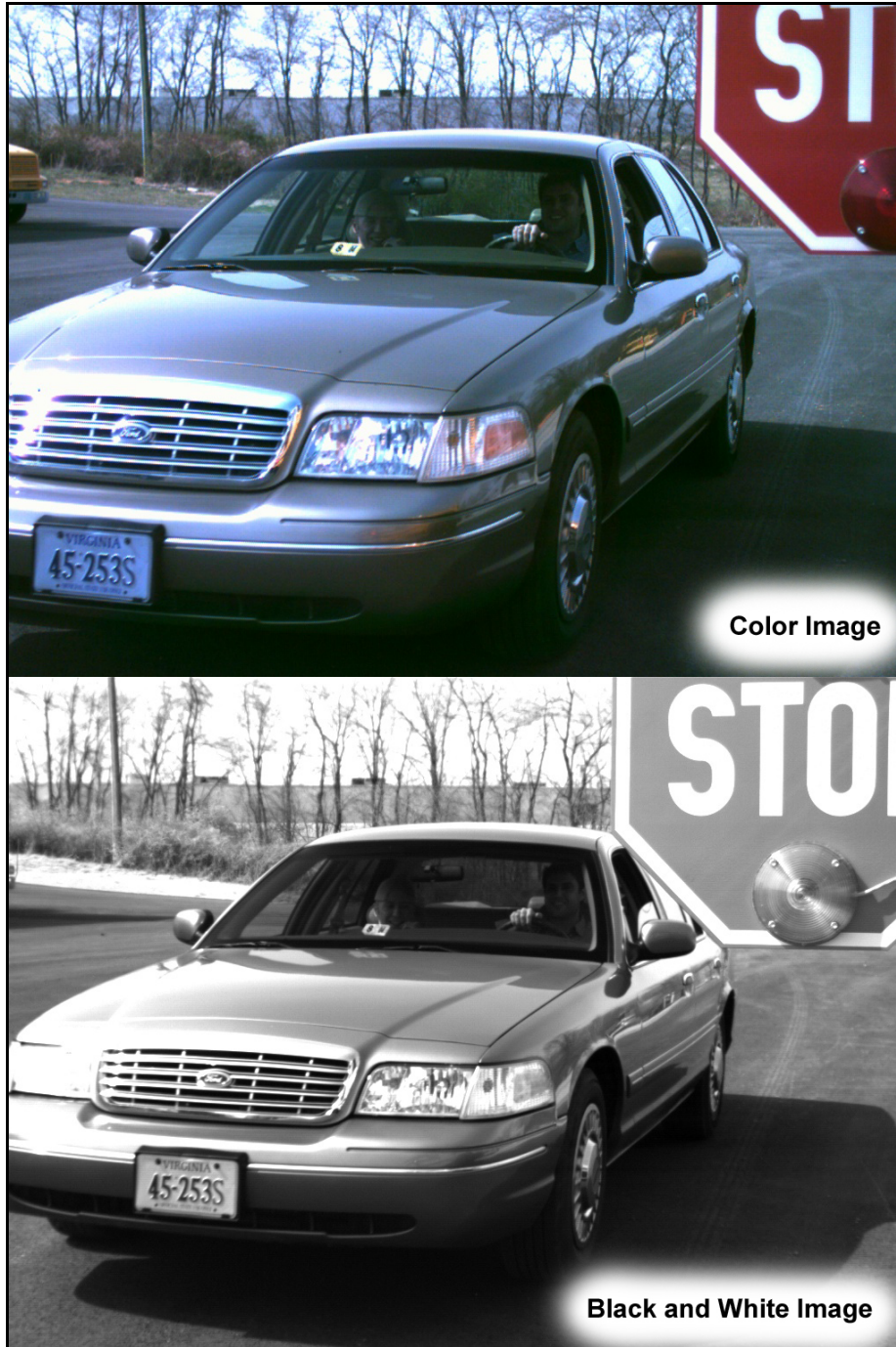
Figure 28. Color and monochrome views from forward-facing cameras (12 mm lens); vehicle is traveling approximately 15 mph.
