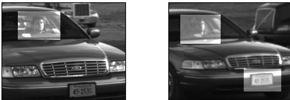
Figure 43. Violating vehicle at 10 feet from system (left picture), and same violating vehicle at 20 feet from the system (right picture). Vehicle is traveling approximately 15 mph.
