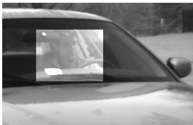
Figure 50. Rain did not noticeably affect facial image quality. Vehicle is traveling approximately 15 mph.
