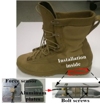
Figure 2.1: The force sensor, aluminum plates, and the installation location.
